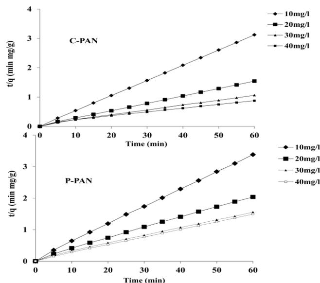
Figure 6: Plot of kinetic data for the adsorption of BB9 onto P-PAN and C-PAN adsorbents
