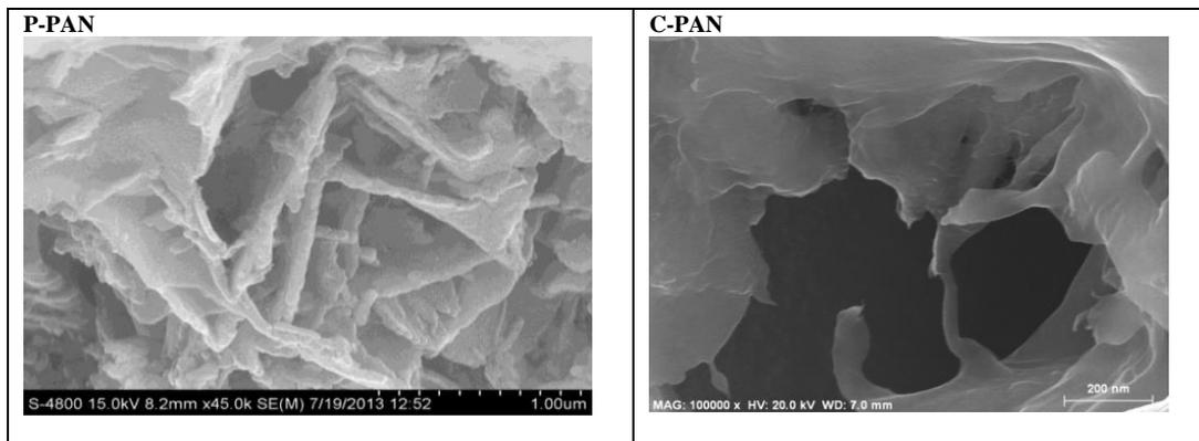
Figure 2: SEM images of C-PAN and P-PAN adsorbents
