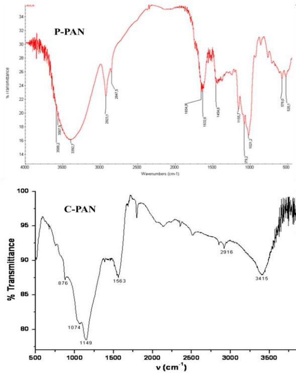
Figure 1: FT-IR spectrum of P-PAN and C-PAN adsorbents
