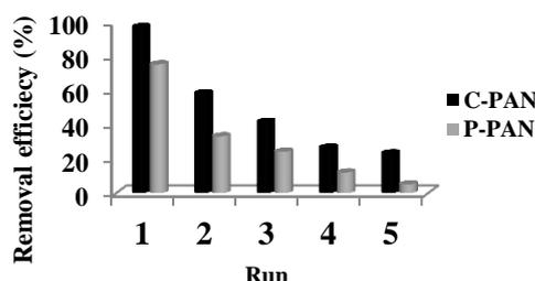
**Figure 7: Reusability of adsorbents: Experimental conditions:  $C_0=20$  mg/l,  $V=50$  ml, ambient temperature and at equilibrium time**
