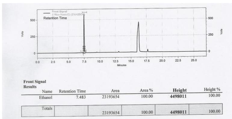
Figure 8: GC graph representing peak of ethanol for 2% H<sub>2</sub>SO<sub>4</sub> pretreated rice husk
