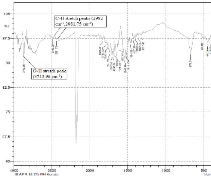
Figure 6: FTIR analysis of acidic pretreated sample after distillation of ethanol
