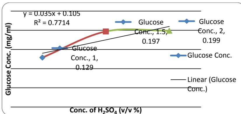
Figure 1: Estimation of reducing sugars after H<sub>2</sub>SO<sub>4</sub> pretreatment
