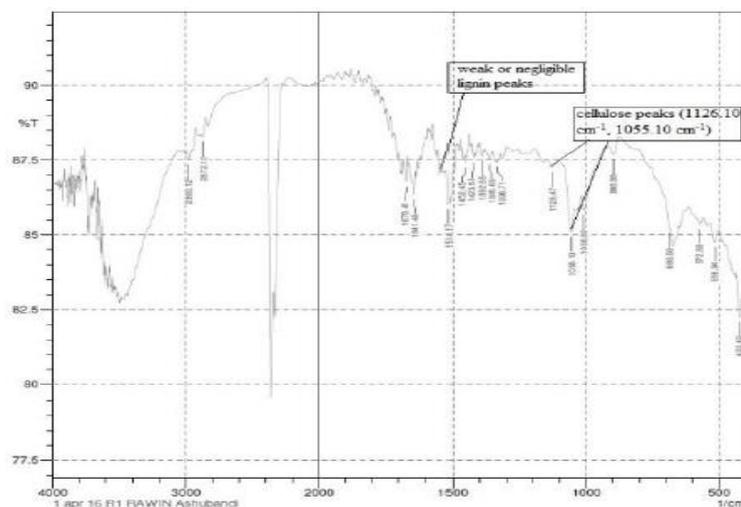
Figure 5: FTIR analysis for alkali pretreated (3% NaOH) sample
