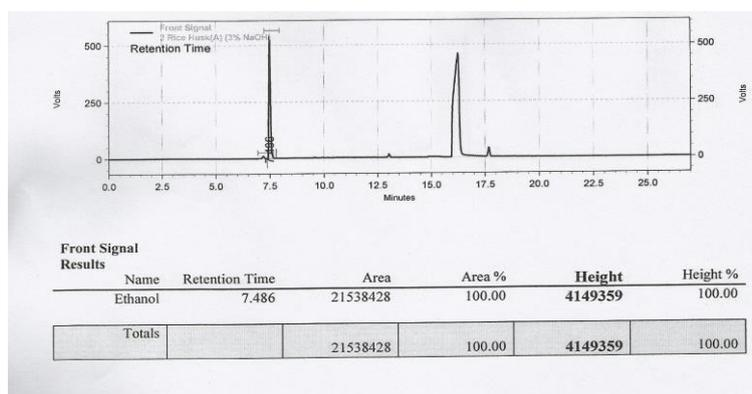
Figure 9: GC graph representing peak of ethanol for 3% NaOH pretreated rice husk
