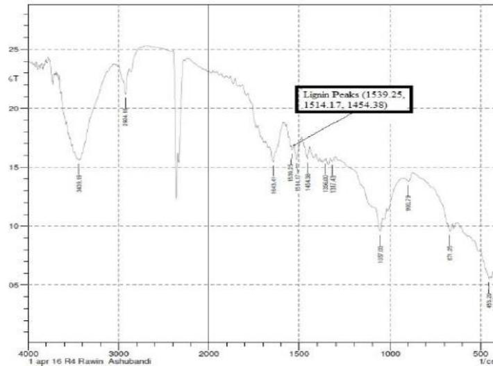
Figure 3: FTIR analysis for untreated rice husk sample
