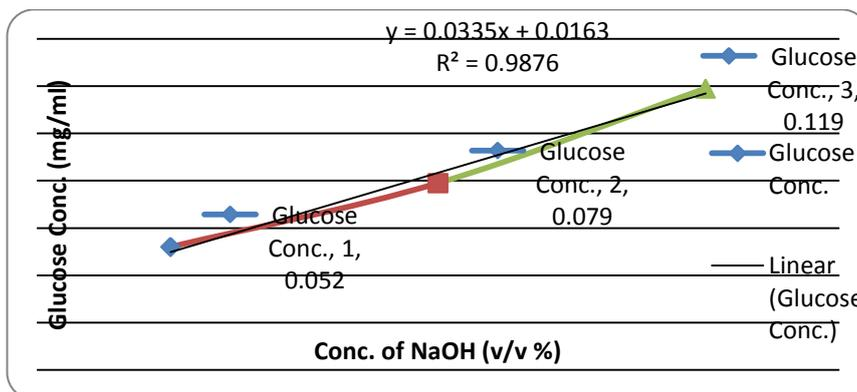
Figure 2: Estimation of reducing sugars after NaOH pretreatment
