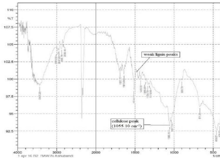
Figure 4: FTIR analysis for acidic pretreated (2% H<sub>2</sub>SO<sub>4</sub>) sample
