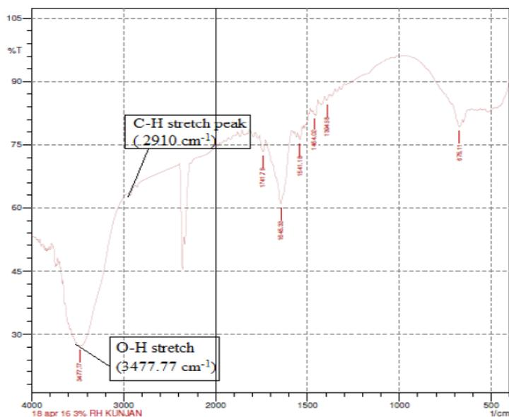
Figure 7: FTIR Analysis of alkali pretreated sample after distillation of ethanol
