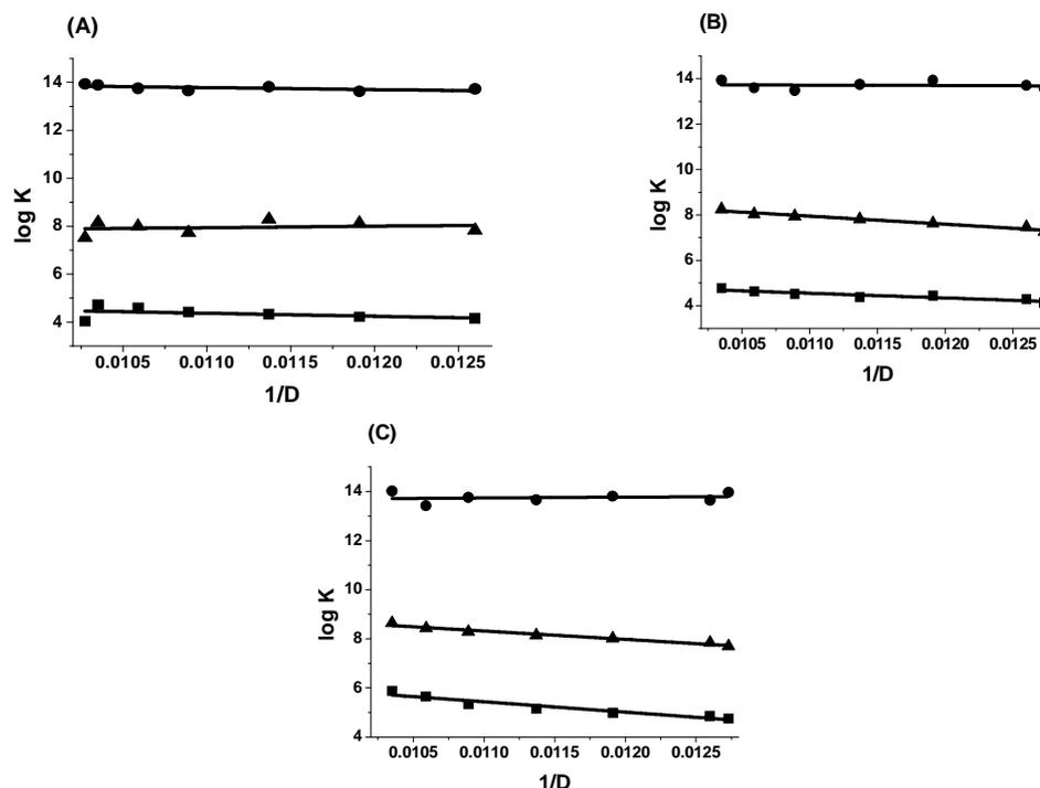
Figure 1. Variation of overall stability constant values of metal-5-SSA complexes with 1/D of Urea-water mixtures (a) Co(II); (b) Ni(II); (c) Cu(II); (■) log  $\beta_{ML}$ ; (▲) log  $\beta_{MLH}$ ; (●) log  $\beta_{ML_2}$ . Distribution Diagrams
