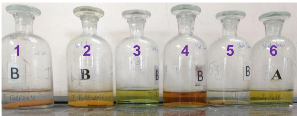
Figure 1: The corrosion of mild steel in different corrosive mediums, (1) water, (2) 0.1 M HCl, (3) 0.01 M CitH<sub>4</sub>-water, (4) 1:1 volume ratio of 0.1 M HCl and 0.01 M CitH<sub>4</sub>, (5) water for 13 days and (6) 0.01 M CitH<sub>4</sub>-water for 13 days
