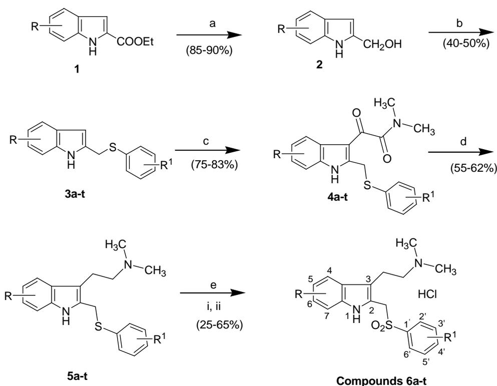
**Reagents and conditions:** a) LiAlH<sub>4</sub>, THF, reflux 3 hr; b) ArSH, THF, p-TSA reflux 3 hr; c) Oxalyl chloride, diethyl ether, RT 1 hr then dimethyl amine aqueous solution (36 %), RT, 2 hr; d) LiAlH<sub>4</sub>, THF, reflux 6 hr; e) i) m-CPBA, CHCl<sub>3</sub>, p-TSA, RT 2.5 hr. ii) IPA.HCl (15 %) 1 hr.
