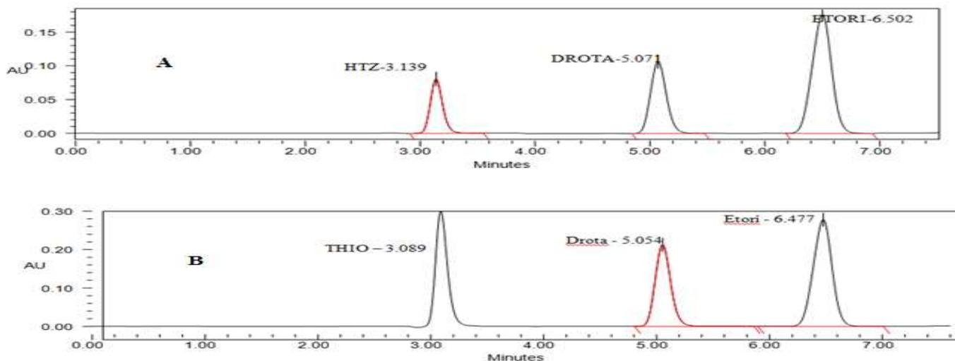
Fig. 4. Chromatogram showing peaks of analytes and internal standards a) Hydrochlorthiazide b) Thiocolchicoside
