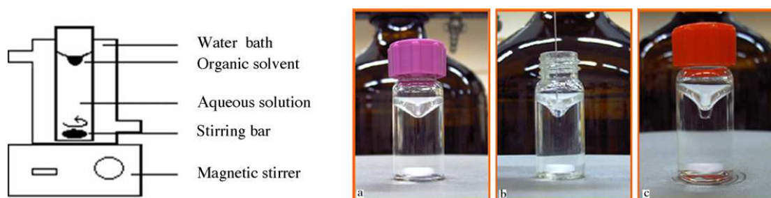
Figure 1. A photograph of the DSDME device.
