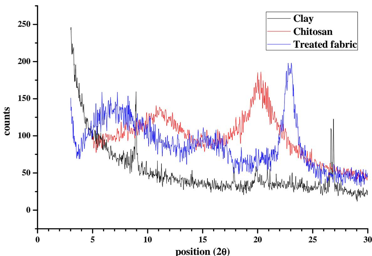
Figure 1 XRD of pure clay (i.e.MMT),pure chitosan (CTS), cotton containing MMT/CTS hybrid nanocomposite
