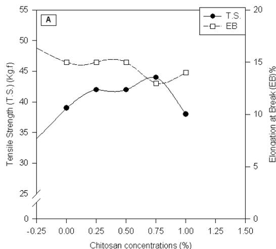
**Figure 5A** Effect of chitosan concentration used in synthesis of MMT/CTS on the tensile strength and elongation at break of fabric treated with the nanocomposite
