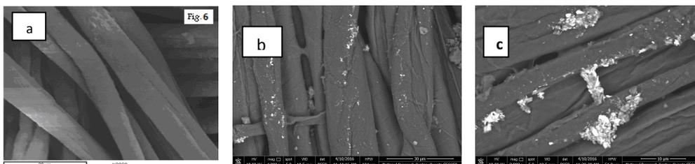
Fig 3 (a-c) SEM of cotton treated with Chitosan/montmorillonite hybrid nanocomposite
