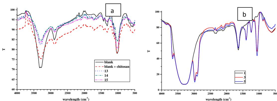
Figure 2 (a,b): FTIR spectra of the cotton fiber and cotton treated with chitosan/montmorillonite hybrid nanocomposite (a); FTIR spectra of chitosan/ montmorillonite nanocomposite prepared using different montmorillonite concentration 1,3,5% (b)
