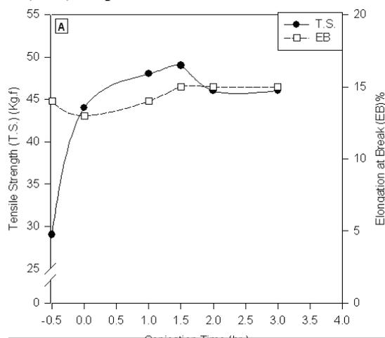
**Figure 7 A Effect of sonication time given for synthesis of MMT/CTS hybrid nanocomposite on the tensile strength and elongation at break of cotton fabric treated with nanocomposite**
