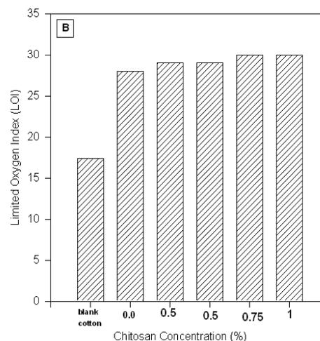
**Figure 5B** Effect of chitosan concentration used in synthesis of MMT/CTS on the tensile Limited Oxygen Limited of fabric treated with the nanocomposite
