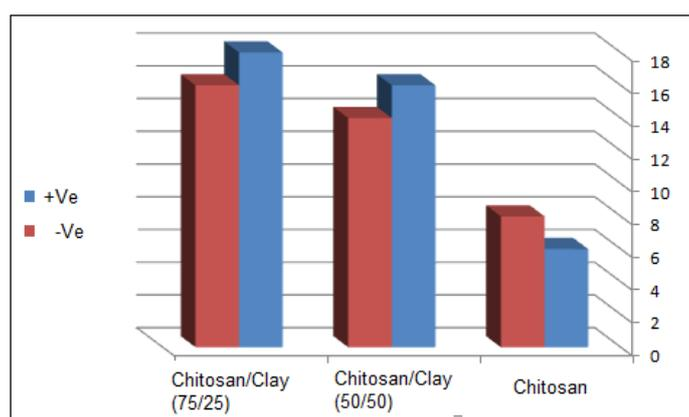
**Fig 9** Reduction percentages of E.coli and S.aureus bacteria of cotton fabric treated with only chitosan vis-à-vis fabric treated with MMT/CTS hybrid nanocomposites using different ratios of MMT:CTS.
