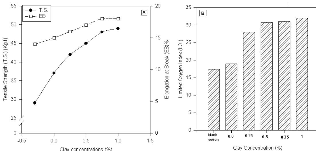
**Figure 6A Effect of MMT concentration used in synthesis of CTS/MMT hybrid nanocomposite on the tensile strength and elongation at break of cotton fabric treated thereof**
