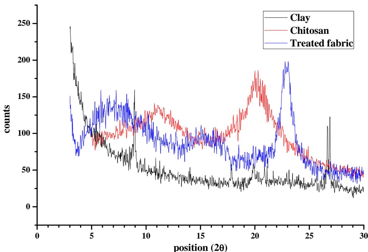
Figure 1 XRD of pure clay (i.e.MMT),pure chitosan (CTS), cotton containing MMT/CTS hybrid nanocomposite
