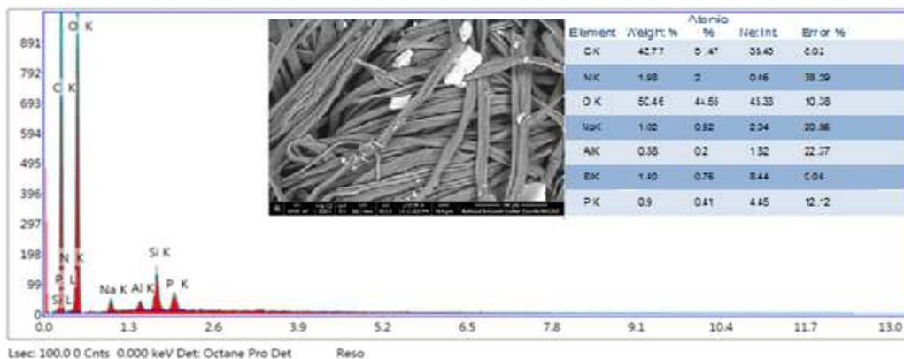
Fig 4 EDX of cotton treated with Chitosan/montmorillonite hybrid nanocomposite
