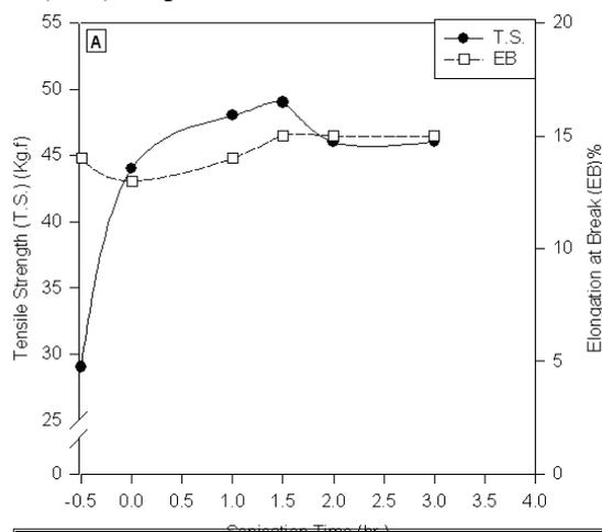
**Figure 7 A Effect of sonication time given for synthesis of MMT/CTS hybrid nanocomposite on the tensile strength and elongation at break of cotton fabric treated with nanocomposite**
