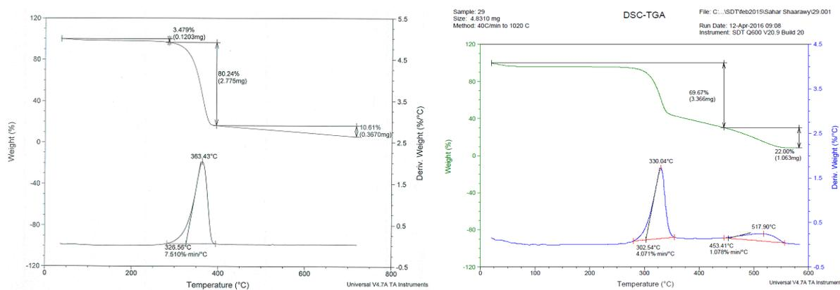
**Figure 8** TGA of untreated cotton fabric and cotton fabric treated with MMT/CTS hybrid nanocomposite concomitantly with citric acid crosslinking catalyzed by SHP
