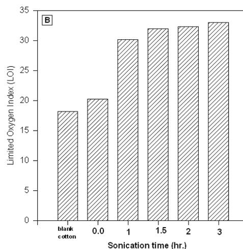
**Figure 7B Effect of sonication time given for synthesis of MMT/CTS hybrid nanocomposite on the Limited Oxygen Index of cotton fabric treated with nanocomposite**
