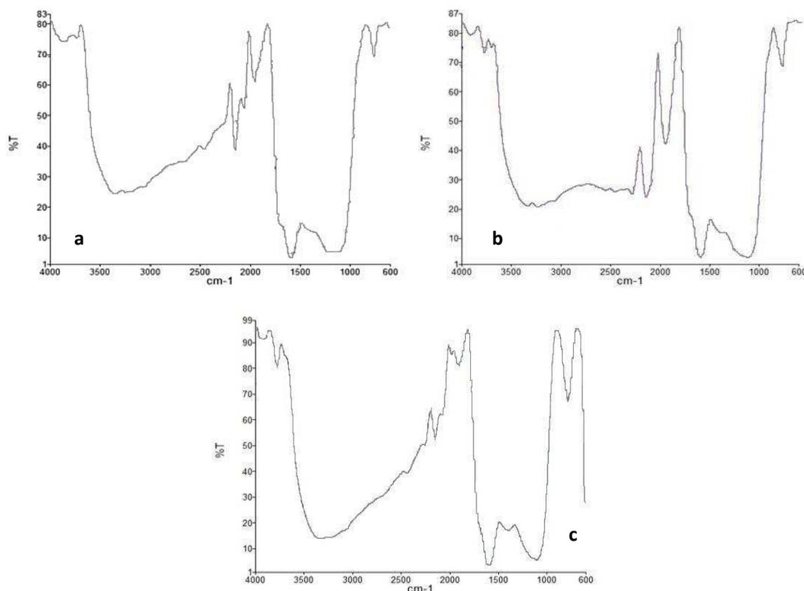
Fig. 4. FT-IR spectra of palm kernel shells carbon (a. 125  $\mu\text{m}$ , b. 90  $\mu\text{m}$ , dan c. 63  $\mu\text{m}$ )
