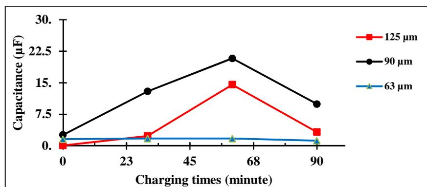
Fig. 5. Effect of carbon particle size of oil palm kernel shell to the capacitance value
