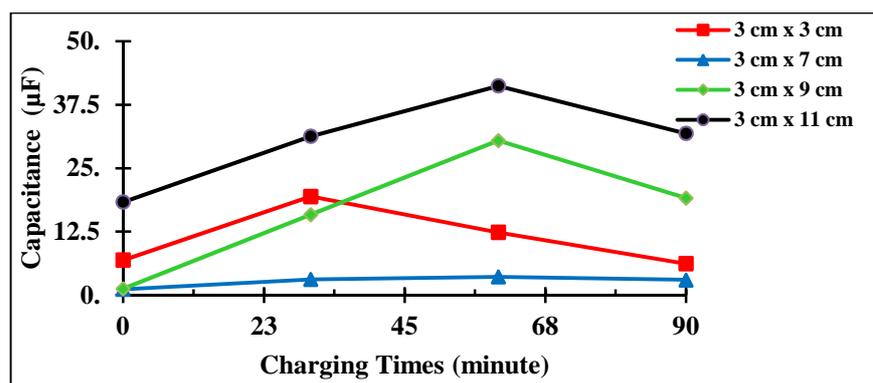
Fig. 6. Effect of carbon paper surface area on the capacitance value
