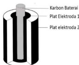
Fig. 1. Schematic illustration of the supercapacitor fabrication
