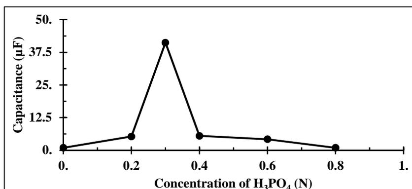
Fig. 8. Effect of  $\text{H}_3\text{PO}_4$  electrolyte concentration against capacitance with charging time of 60 minutes
