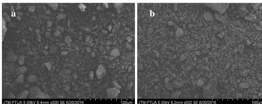
Fig. 3. SEM image of palm kernel shells carbon with a combustion temperature (a.) 300°C (b.) 400°C
