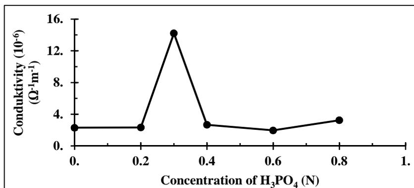
Fig. 9. Effect of  $H_3PO_4$  electrolyte concentration on the conductivity
