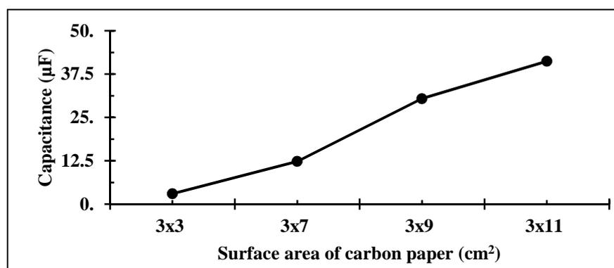
Fig. 7. Effect of surface area of carbon paper on capacitance on the charging time of 60 minutes
