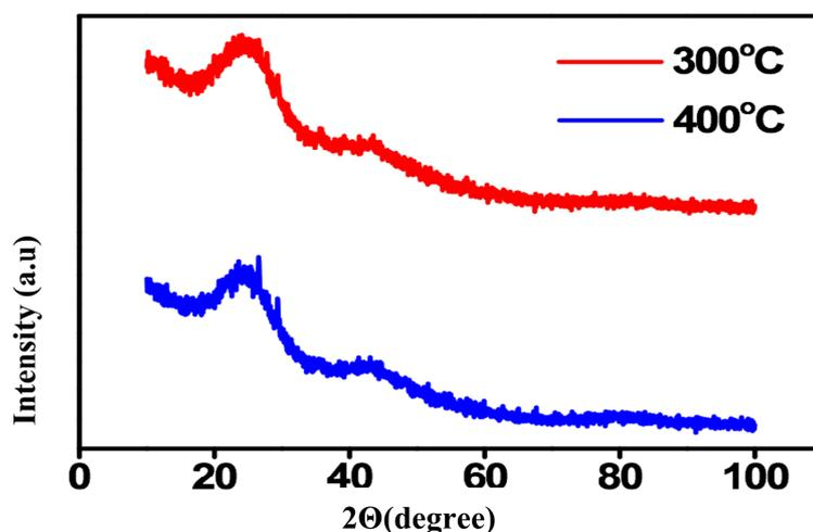
Fig. 2. XRD pattern of oil palm kernel shell carbon with a combustion temperature at 300°C and 400°C
