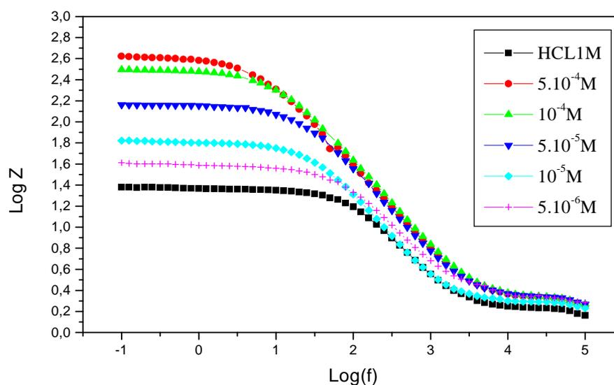
**Fig. 1.b Bode diagrams for steel in 1M HCl containing different concentrations of P4.**
