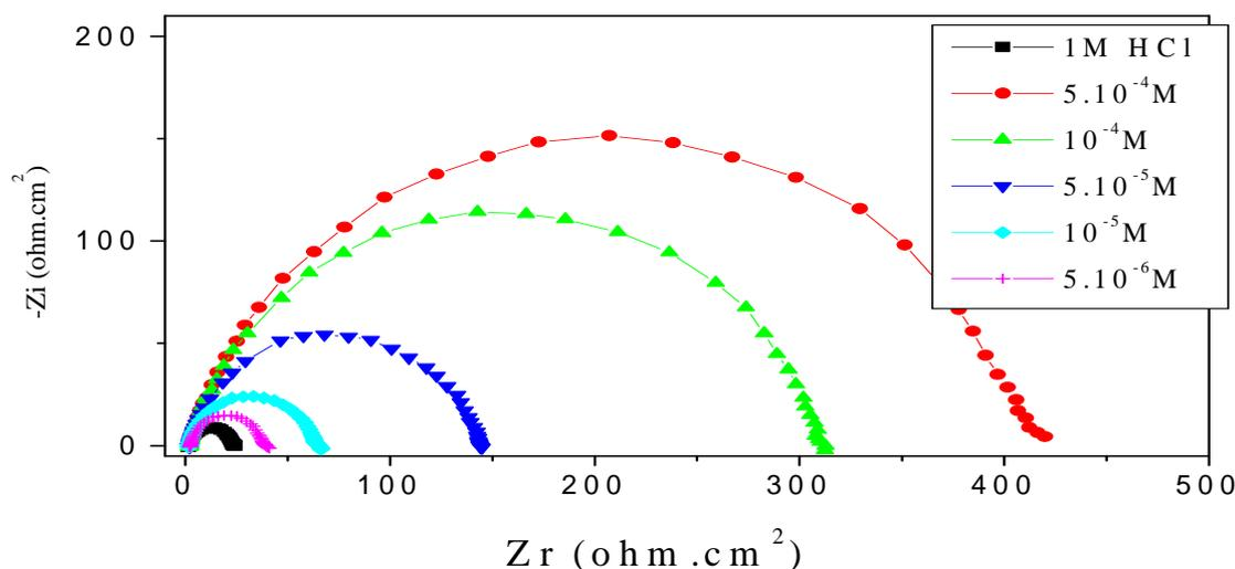
Fig. 1a. Nyquist plots of steel in 1M HCl containing various concentrations of P4 at  $E_{\text{corr}}$ .
