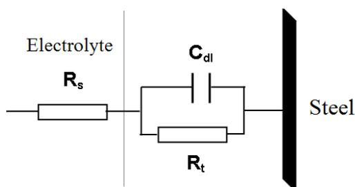
Fig. 1.c Electrochemical equivalent circuit diagram for metal–electrolyte interface.
