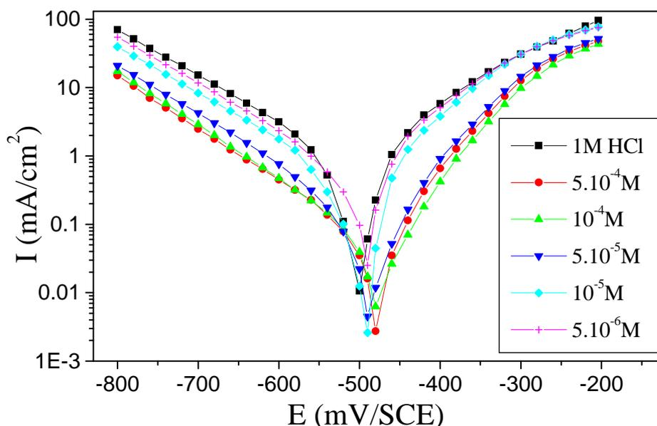
Fig. 2. Polarisation curves of steel in 1M HCl for various concentrations of P4
