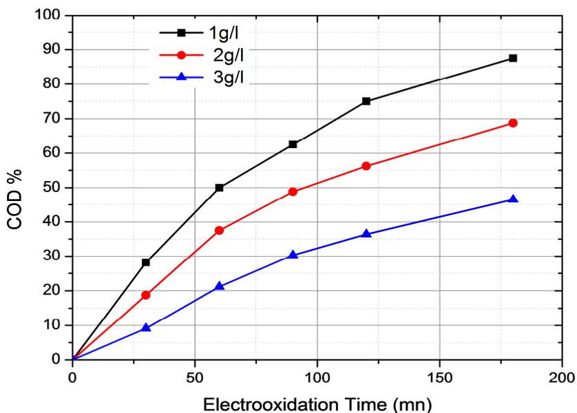
Fig. 8. Direct electrooxidation at BDD anode: effect of initial concentration of thiabendazole on the %COD ( $80\text{ mA}\cdot\text{cm}^{-2}$ , and  $T=25^\circ\text{C}$ )
