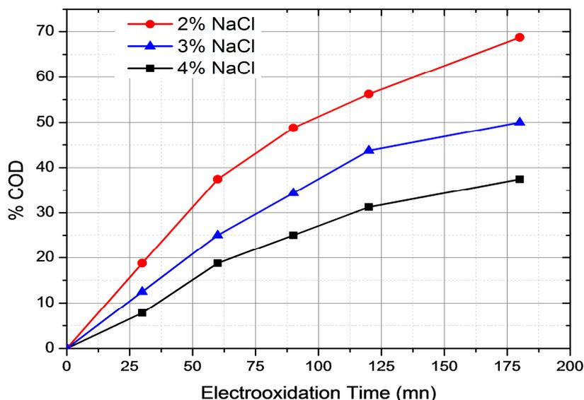
**Fig. 2.** Influence of supporting electrolytes on the decay of COD during electro-oxidation of 1680 mg/L thiabendazole on BDD anode. Conditions: Current density 60 A.cm<sup>2</sup>; T: 25°C
