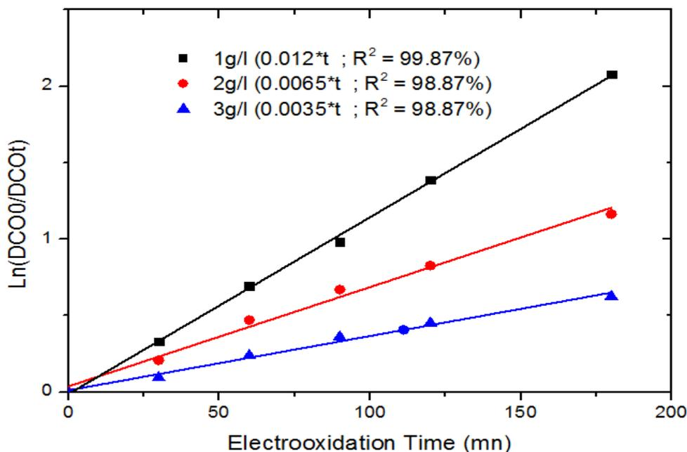
Fig. 9. Pseudo first-order plot oxidation of thiabendazole:  $T= 25^\circ\text{C}$ , 2% NaCl at  $80\text{ mA}\cdot\text{cm}^{-2}$ , for different concentration
