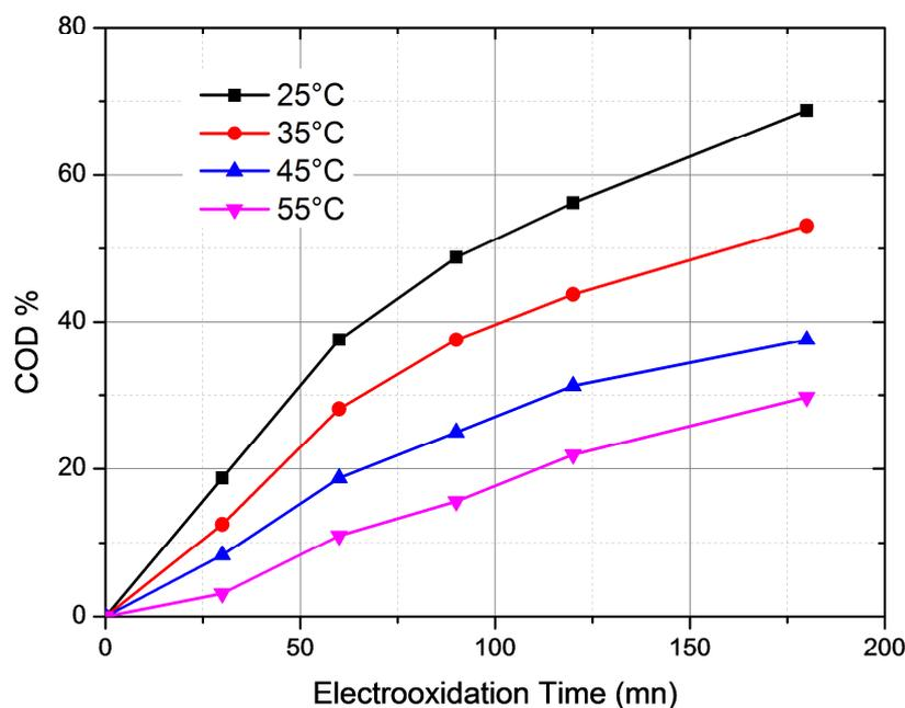
Fig. 6. % COD reduction for thiabendazole in 2% NaCl at 25°C and volume of treated solution: 75 cm<sup>3</sup> at different temperatures, 80 mA
