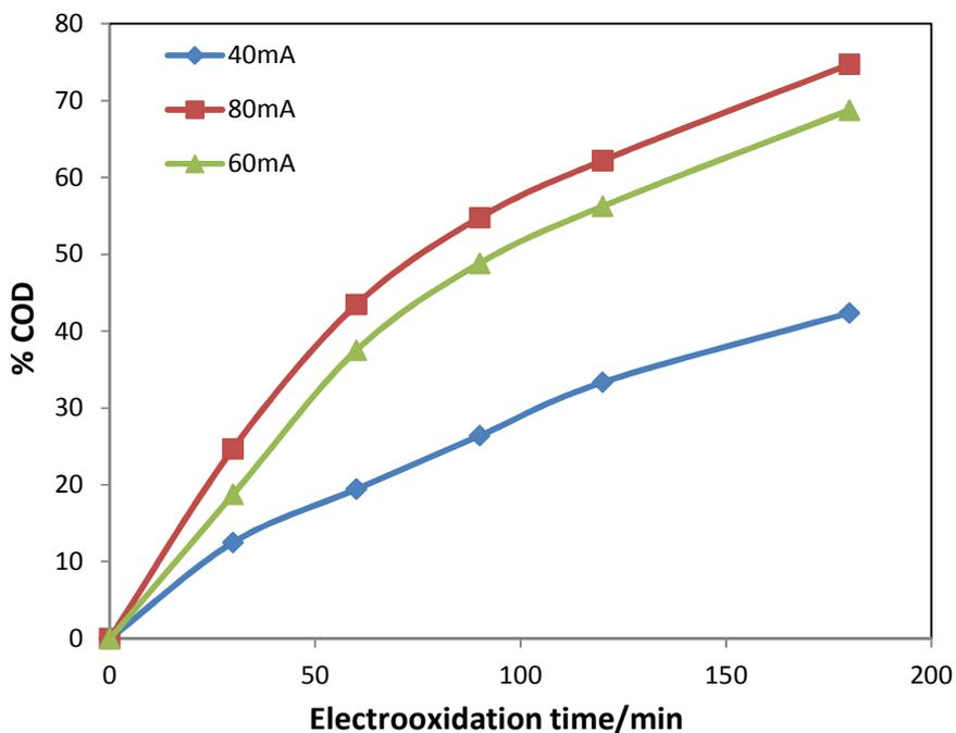
Fig. 4. Influence of the applied current density on the trends of % COD electrolysis of Thiabendazole ( $COD_0 = 1680 \text{ mg.L}^{-1}$ ) using a  $1 \text{ cm}^2$  BDD anode
