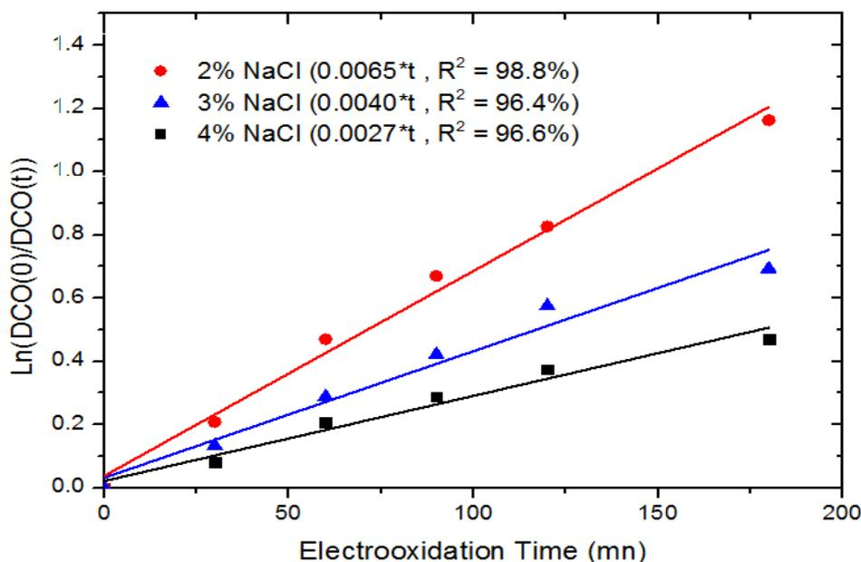
Fig. 3. Pseudo first-order plot oxidation of 2g/L thiabendazole ( $\text{COD}_0 = 1680 \text{ mg/L}$ ) in different concentration of electrolyte at  $60 \text{ mA.cm}^{-2}$
