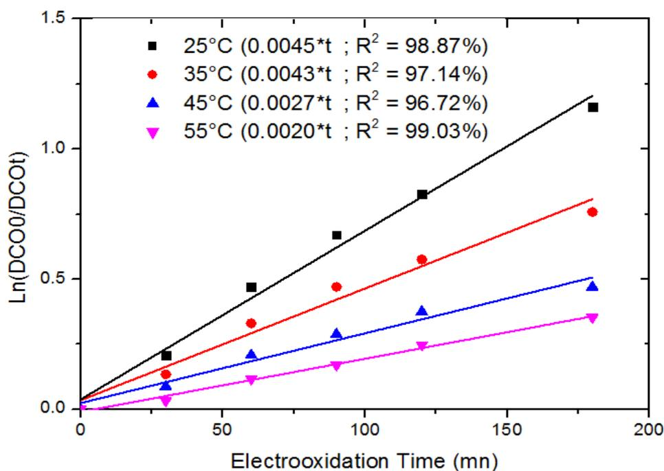
Fig. 7. Pseudo first-order plot oxidation of thiabendazole in 2% NaCl at 80 mA and volume of treated solution: 75 cm<sup>3</sup> under different temperatures (COD at a given time, t, during electrolysis)
