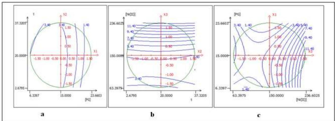
Figure 7: Isoresponse curves adsorption of nickel (II) on phosphogypsum: (a) Effect of adsorbent dosage and contact time ([Ni (II)] initial=150 mg/l); (b) Effect of contact time and initial Ni(II) concentration ([PG]=15 g/l); (c) Effect of initial Ni(II) concentration and adsorbent dosage on the amount of nickel (mg/g) (t=20 min)
