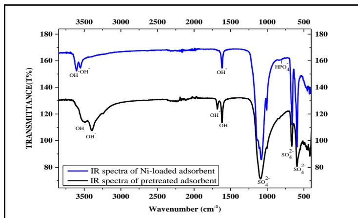
Figure 1: Infrared spectra of adsorbent before and after adsorption of nickel ions
