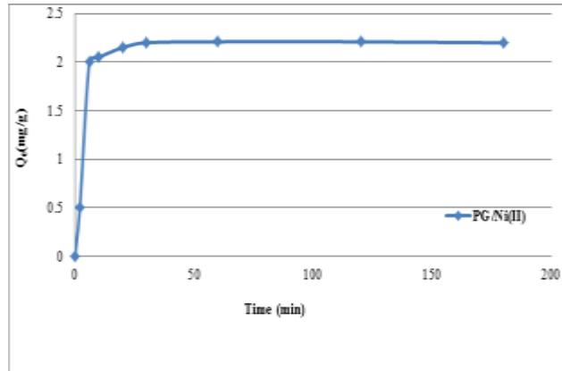
Figure 3: Effect of initial contact time (Initial concentration of Ni(II), 200 mg/l; phosphogypsum dosage, 2 g/100 ml; pH 7.01)
