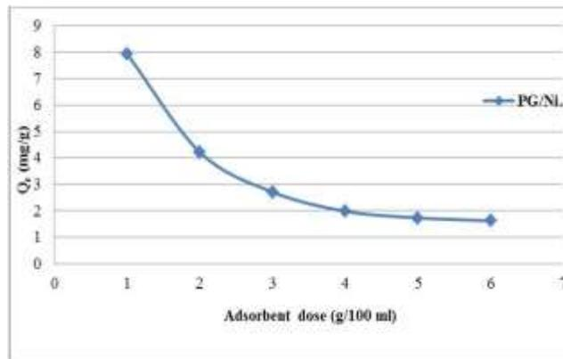
Figure 4: Effect of phosphogypsum dosage (Initial concentration of Ni(II), 200 mg/l; Contact time: 40 min, Ph 7.01)
