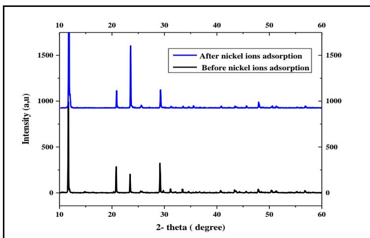
Figure 2: X-ray diffraction patterns of adsorbent before and after the adsorption process
