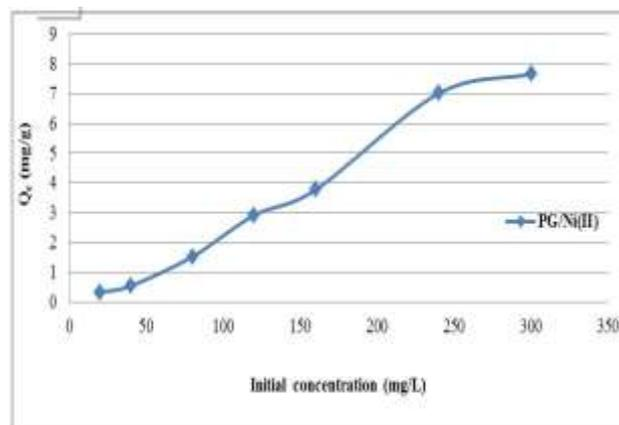
Figure 5: Effect of initial Ni(II) concentration (phosphogypsum dosage, 2 g/100 ml; Contact time: 40 min, pH 7.01)
