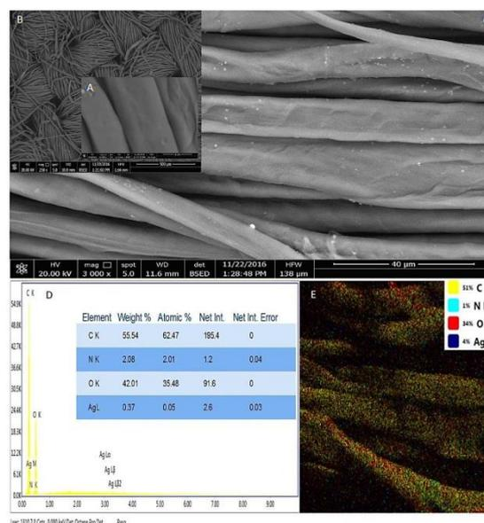
**Figure 4: SEM image (A) Untreated cotton fabrics with AgNPs; (B and C) Treated cotton fabrics with AgNPs; (D) EDX of treated sample with elemental analysis of the AgNPs contents and; (E) Mapping picture of the surface of treated fabrics with AgNPs**
