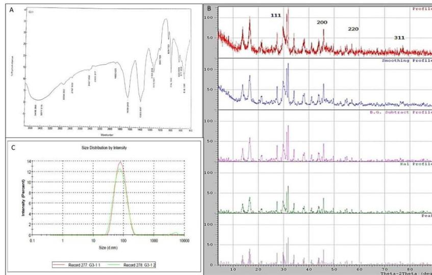
**Figure 3: (A) FTIR spectra showing the presence of proteins as capping agents for AgNPs synthesized by *Aspergillus niger* G3-1; (B) XRD pattern of silver nanoparticles synthesized by *Aspergillus niger* G3-1; (C) Particle size distribution for silver nanoparticles synthesized by *Aspergillus niger* G3-1**
