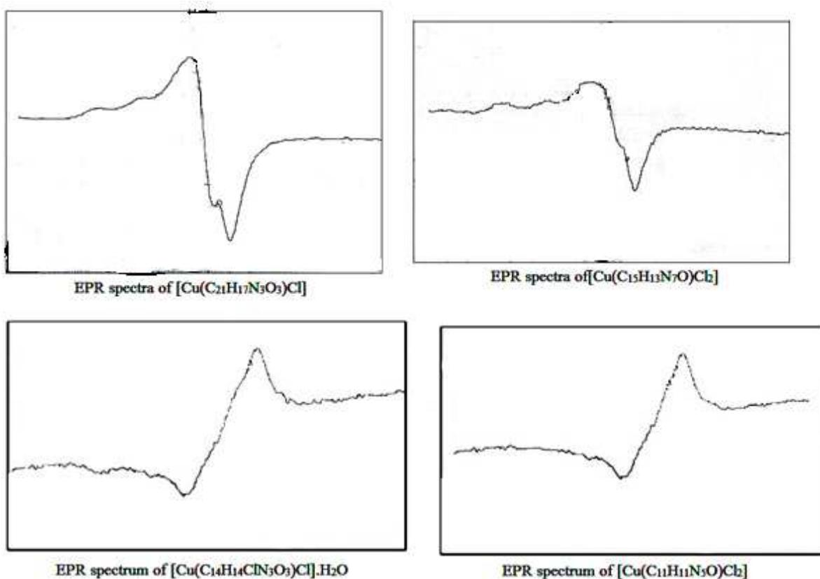
Figure-3: EPR spectra of investigated Cu(II) complexes
