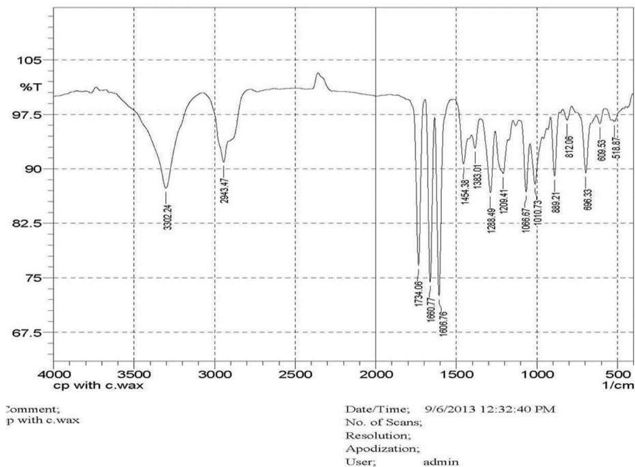
Figure 2: IR Spectra of clobetasol propionate with carnauba wax
