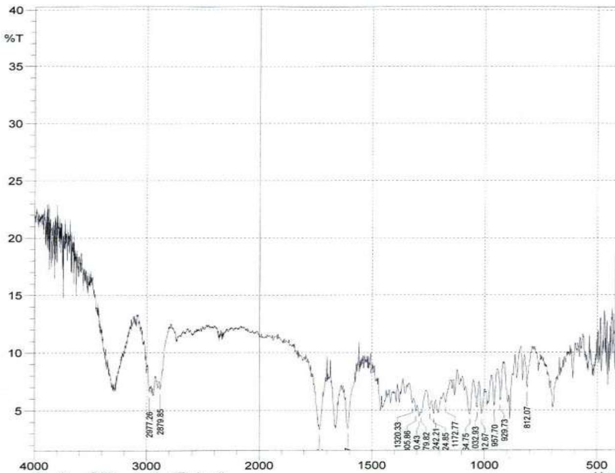
Figure 1: IR Spectra of clobetasol propionate
