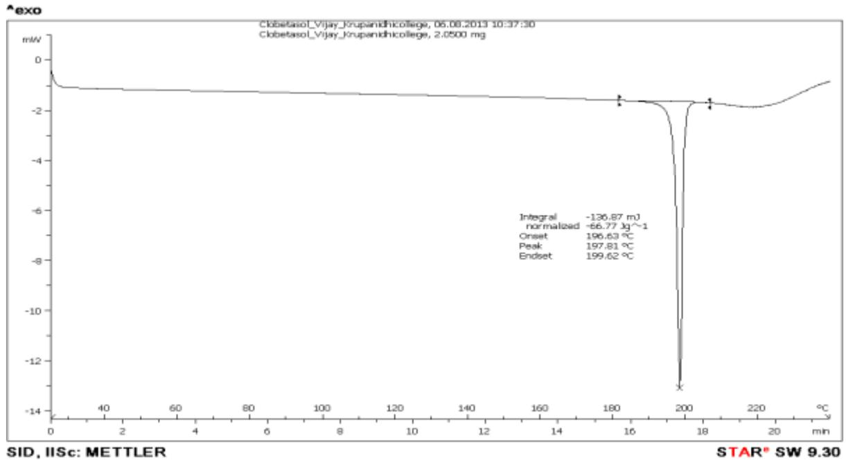
Figure 3: DSC thermogram of clobetasol propionate
