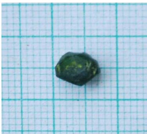
Fig.1. As grown crystal of NBTN single crystal
