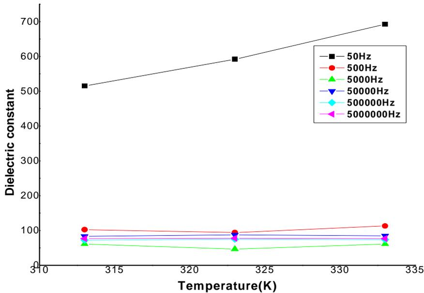
Fig.4.Dielectric constant of NBTN crystal with log frequency
