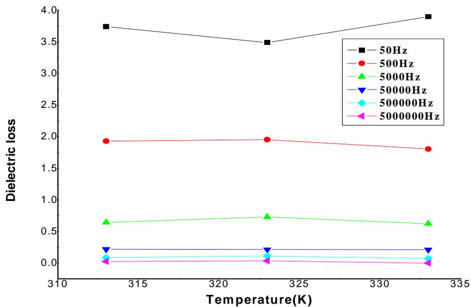
Fig.5. Dielectric loss of NBTN with log frequency
