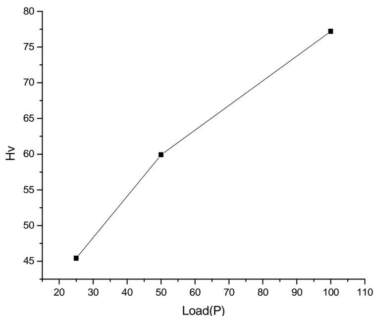
Fig.6. Microhardness Curve of NBTN crystal
