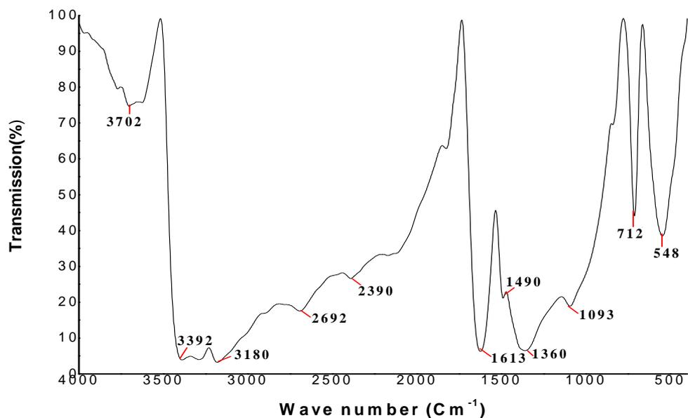
Fig .2.FTIR spectrum of NBTN single crystal
