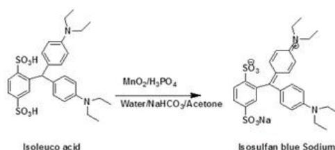
Figure 1: Reaction scheme for the synthesis of isosulfanblue blue
