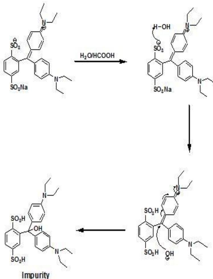
Figure 7: Mechanism for the formation of impurity 1
