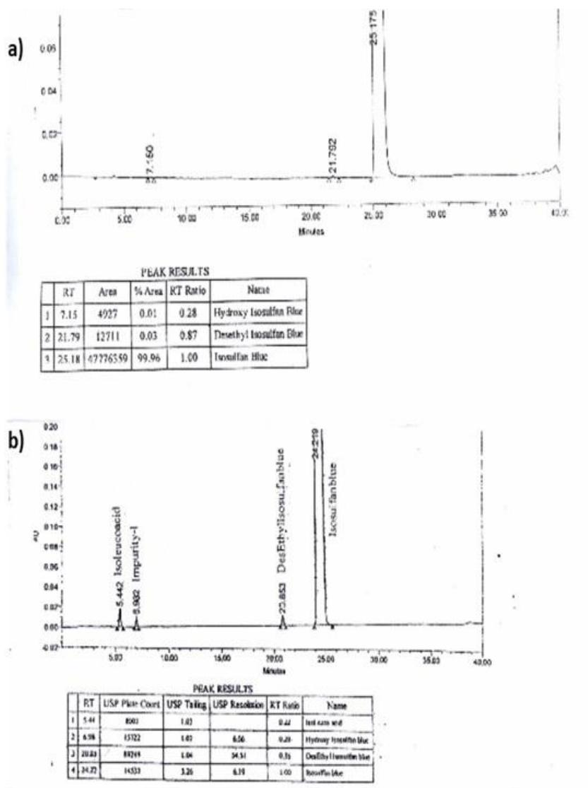
Figure 4: HPLC chromatogram of (a) Isosulfanblue and its impurities, (b) Isosulfanblue sample spiked with impurities
