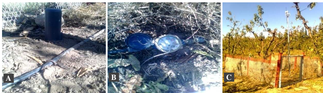
Fig. 2: Measuring tools used in the experiment: (A) Soil moisture sensor FDR, (B) Pulse flow meter, (C) Telemetry system and transmission unit
