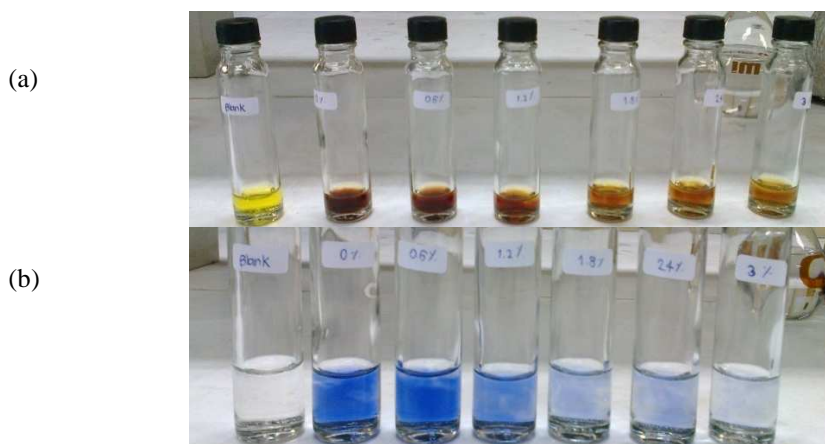
Figure (5): The color shades of the reaction products using 0.06 mg/L cyanide with red solution (a) and blue solution (b) in the presence of propanol concentrations of 0, 0.6, 1.2, 1.8, 2.4 and 3.0 % (v/v)
