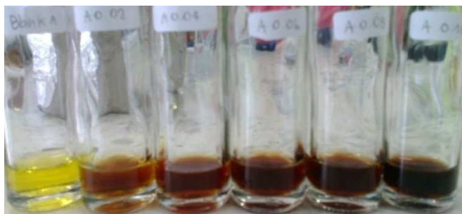
Figure (2): The reaction product of ninhydrin in the presence of cyanide concentrations of 0.0, 0.02, 0.04, 0.06, 0.08 and 0.10 mg/L in sodium carbonate solution (red solution)
