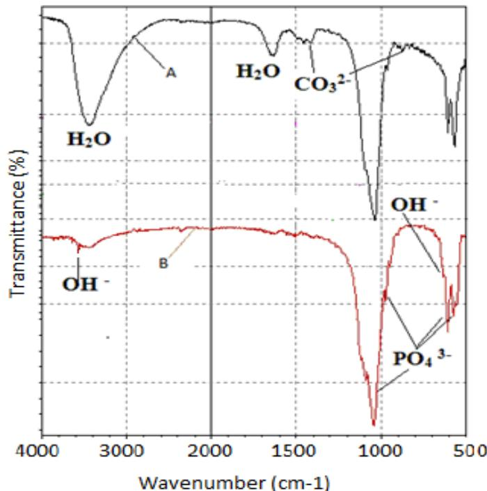
Figure 1. Fourier-transformed infrared spectroscopy of apatite prepared
