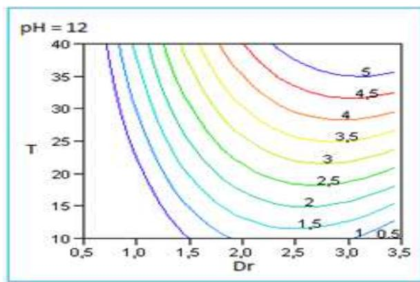
**Figure 7.** isoresponse plot of %O<sub>2</sub> in (Dr, T) plan with pH fixed at 12.
