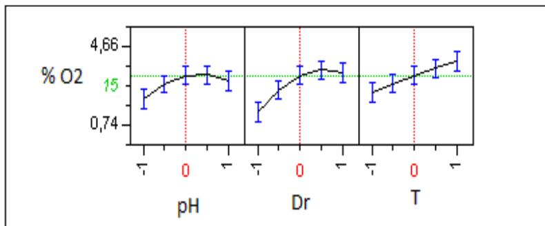
Figure 4. Main effects plot for % O<sub>2</sub> inserted
