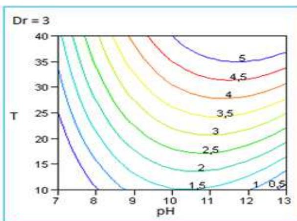
**Figure 8.** isoresponse plot of %O<sub>2</sub> in (pH, T) plan with Dr fixed at 3 days.
