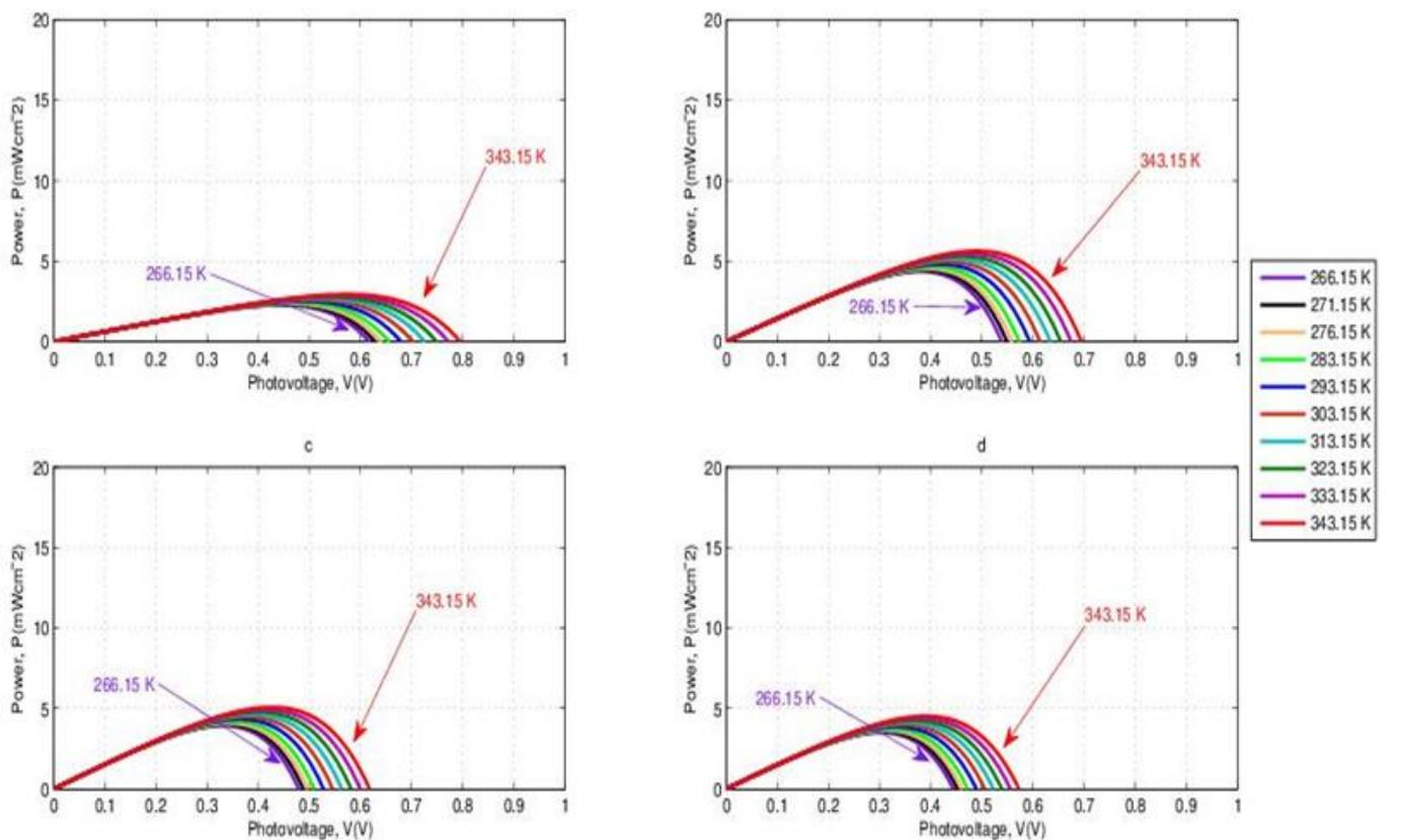
Figure 2: Variation of the power under different temperature and various thin film electrode thicknesses: (a) 1 μm, (b) 5 μm, (c) 10 μm and (d) 15 μm
