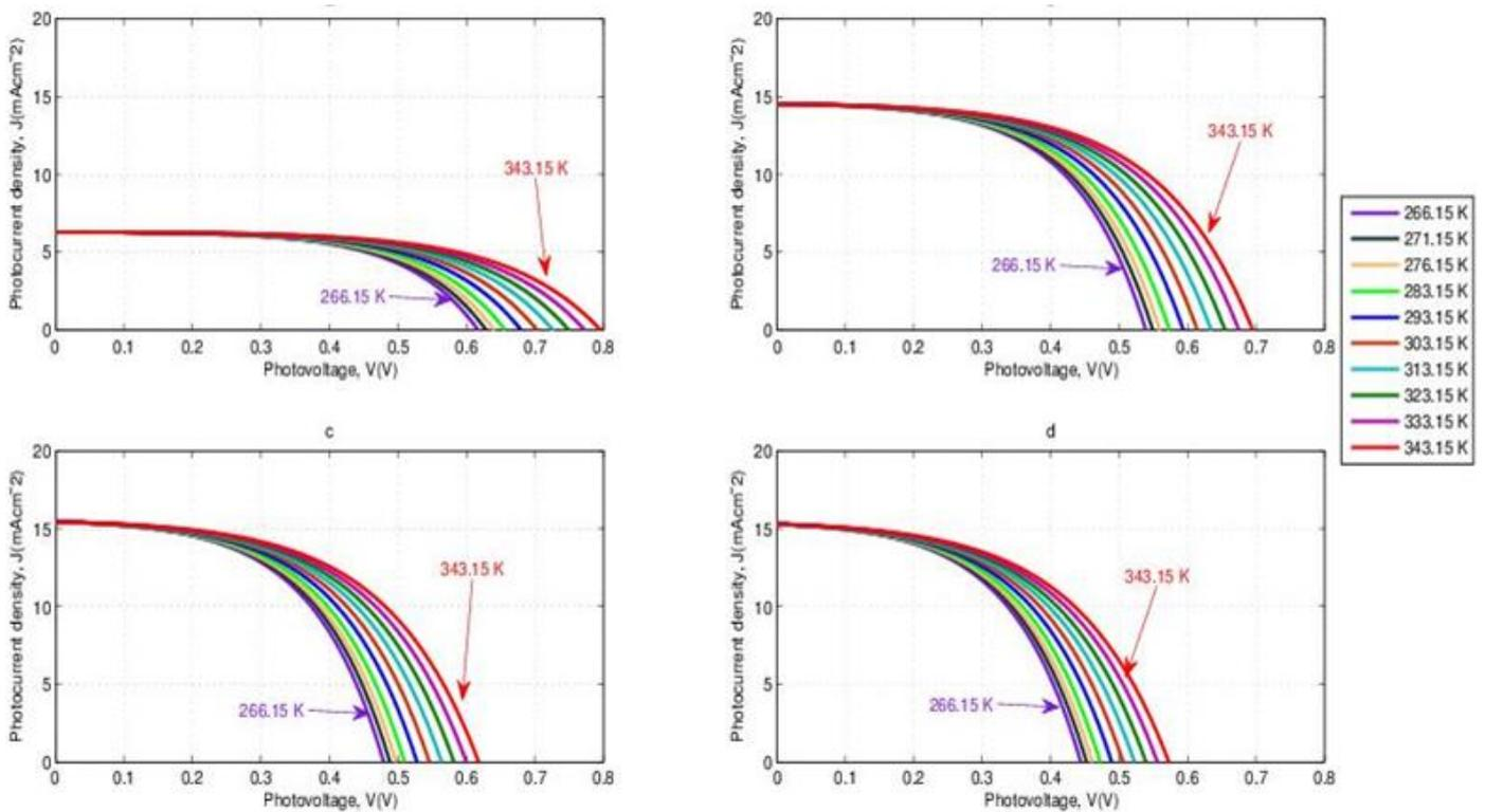
Figure 1: Variation of the DSSCs J-V characteristics under different temperature and various thin film electrode thicknesses: (a) 1 μm, (b) 5 μm, (c) 10 μm and (d) 15 μm
