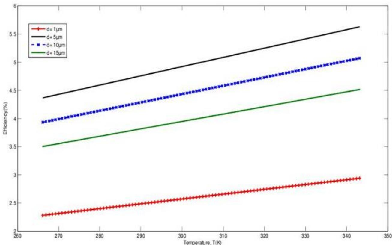
Figure 3: The effect of temperature on conversion efficiency with different thickness of the electrode
