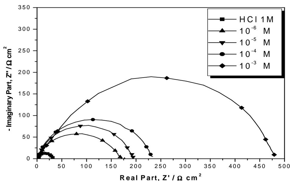
**Figure 2: Nyquist plots of mild steel in 1 M HCl containing different concentrations of BDIP**
