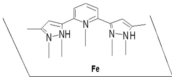
**Scheme 2: Schematic representation of the mode of adsorption of BDIP onto the mild steel surface**
