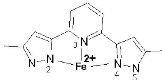
**Scheme 3: Complex suggested to be formed on the mild steel surface**
