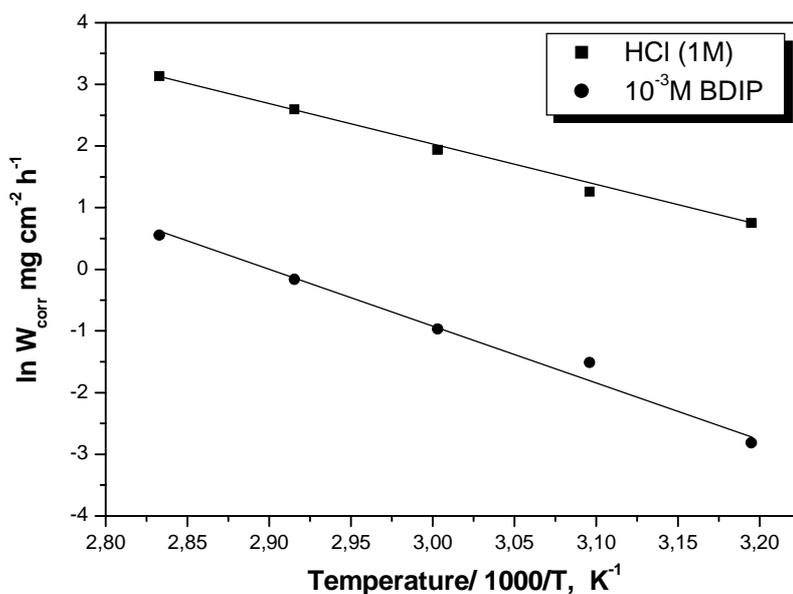
Figure 3: Arrhenius plots for  $\ln W_{corr}$  vs.  $1/T$  for mild steel in 1 M HCl at  $10^{-3}$  M of BDIP
