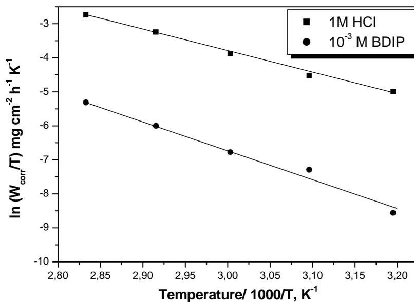
Figure 4: The relation between  $\ln (W_{corr}/T)$  vs.  $1/T$  for mild steel at  $10^{-3}$  M of BDIP
