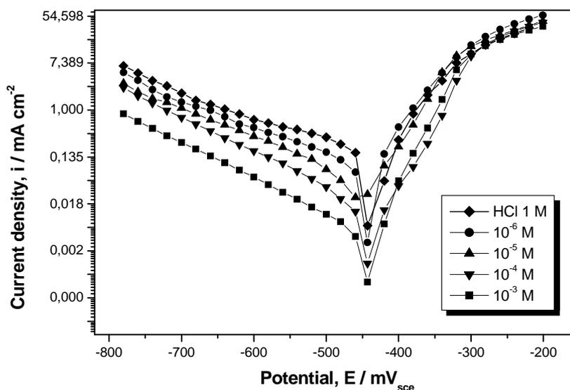
**Figure 1: Cathodic and anodic plots of mild steel in 1 M HCl at different concentrations of BDIP**
