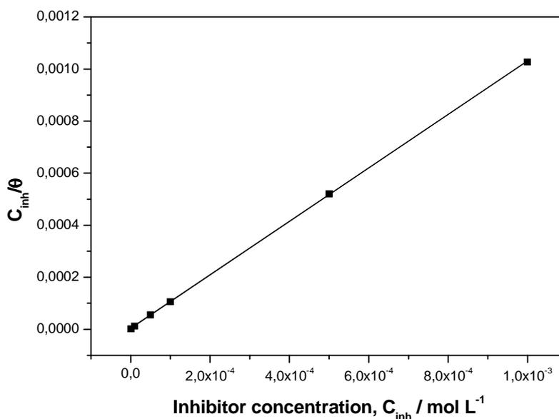
Figure 5: Langmuir isotherm adsorption model of BDIP on the surface of mild steel in 1 M HCl
