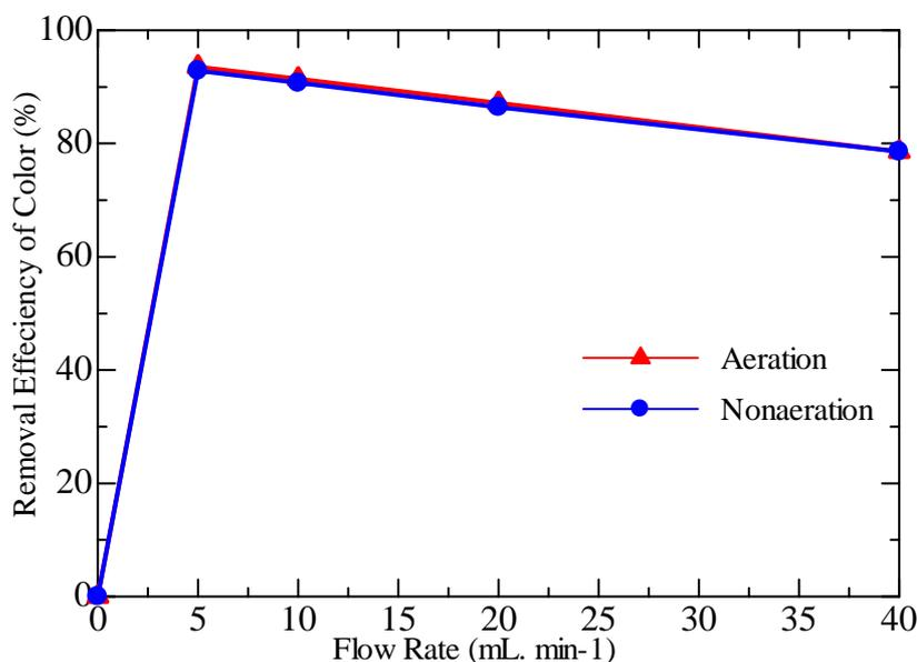
Fig. 3. Removal efficiency of color of peat water
