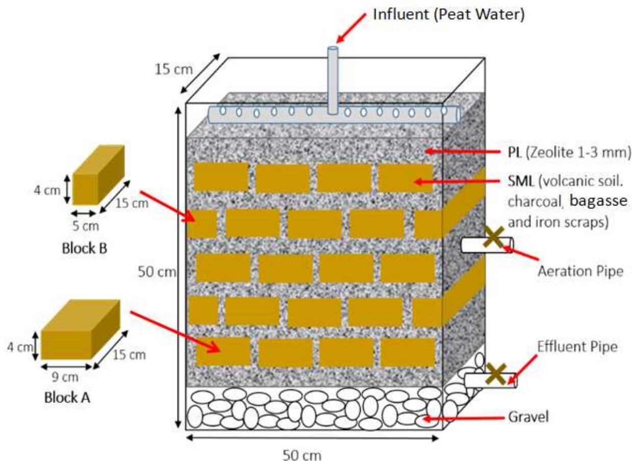
Fig. 1.Design of MSL system
