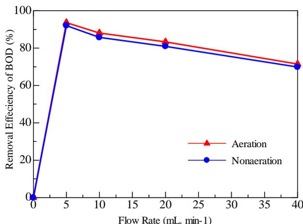
Fig. 5. removal efficiency of BOD of peat water
