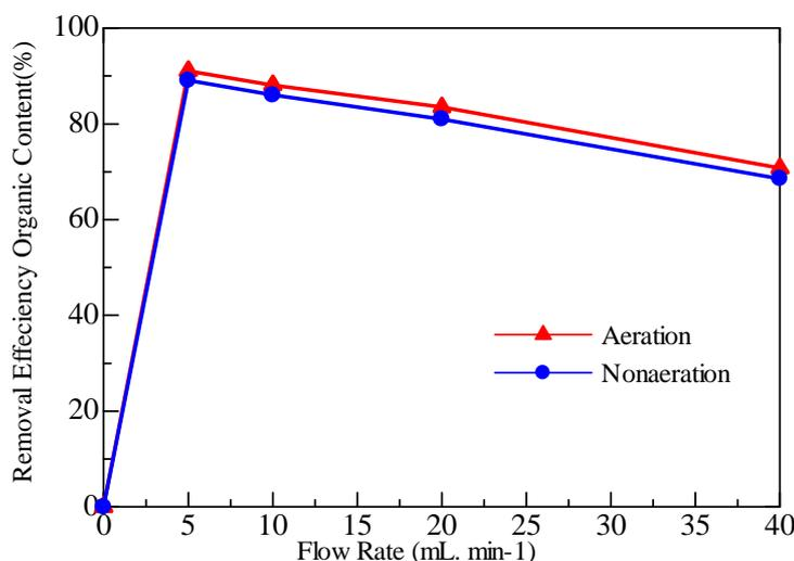
Fig. 6. Removal efficiency of organic content of peat water
