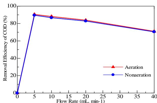
Fig. 4. Removal efficiency of COD of peat water
