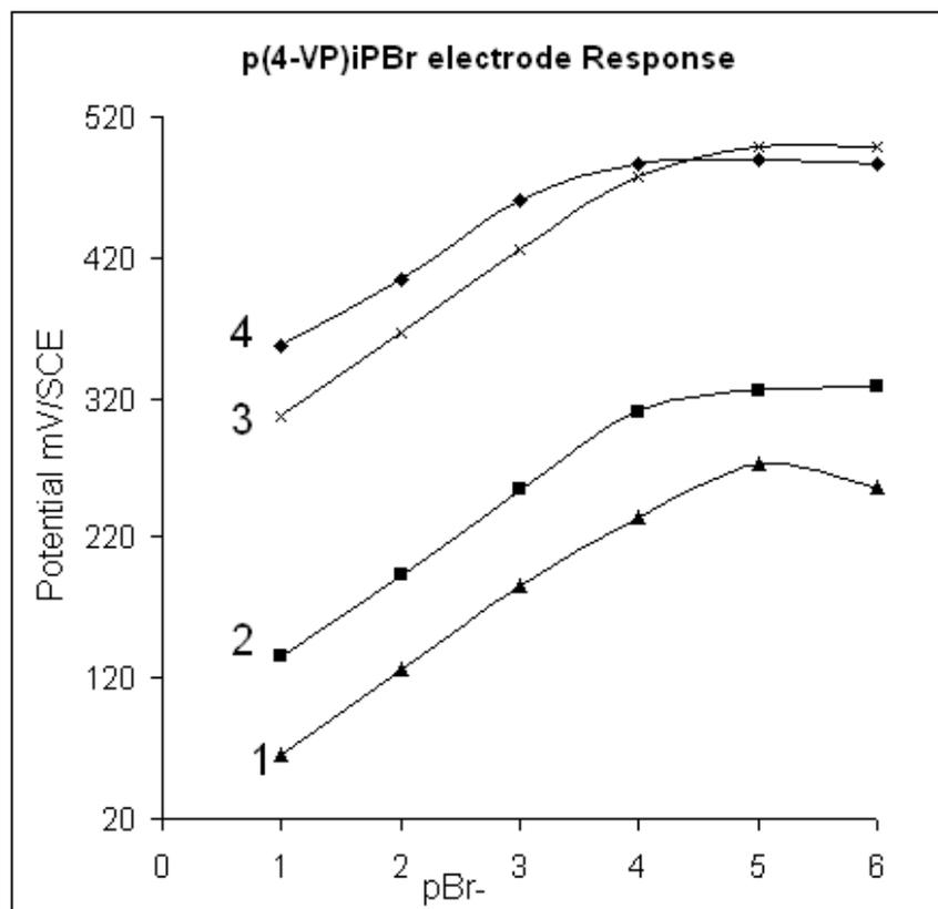
**Fig.3. Response electrode in bromide solution at various pH**
