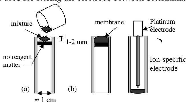
**Fig. 2. Preparation of selective electrode**
