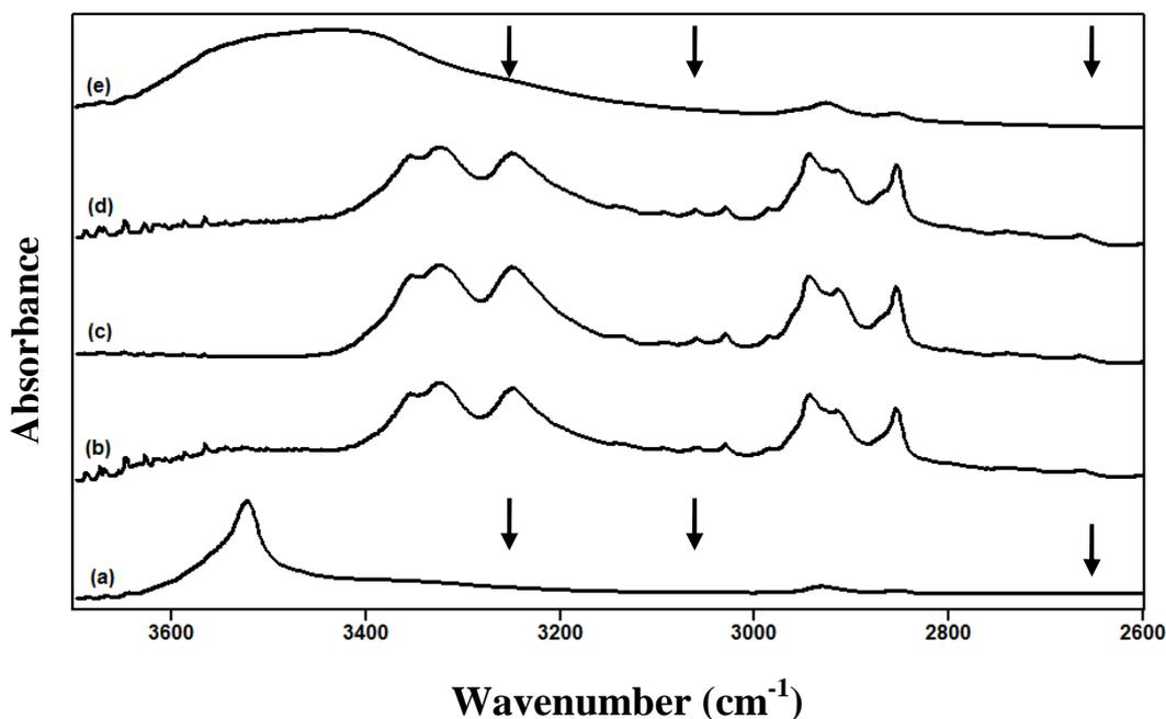
Figure 2a: The FTIR spectra of (a) GPZ-Cd(II) in 2:1 ratio, (b) GPZ-Cd(II) in 1:1 ratio, (c) pure GPZ, (d) GPZ-Ni(II) in 1:1 ratio, and (e) GPZ-Ni(II) in 2:1 ratio in the region of 2600-3700 cm<sup>-1</sup>
