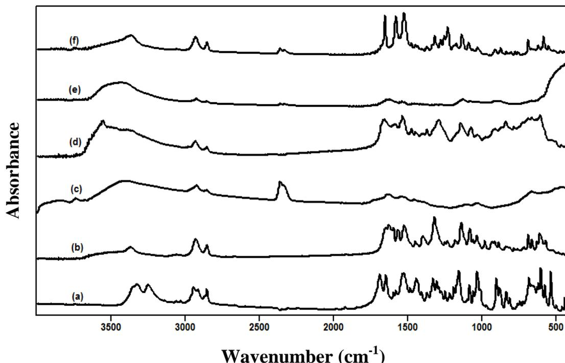
Figure 3: The FTIR spectra of (a) pure GPZ, (b) GPZ-Hg(II), (c) GPZ-Fe(III), (d) GPZ-Co(II), (e) GPZ-Zn(II) and (f) GPZ-Ca(II) in 2:1 ratio in the region of 400-4000  $\text{cm}^{-1}$
