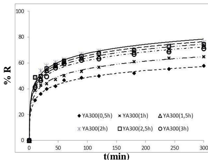
**Fig 3.** adsorption kinetics of MB molecule by YA300t (t: the activation time)
