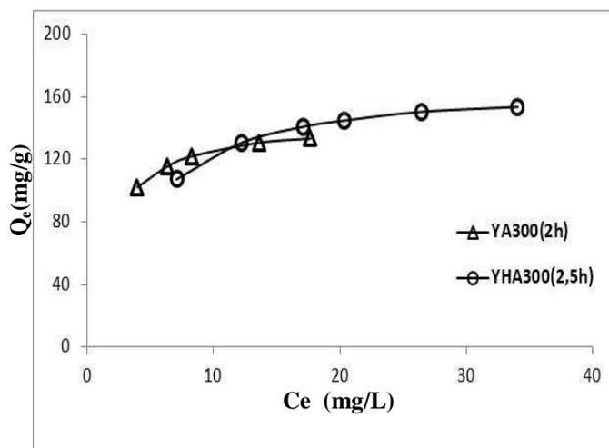
**Fig 8. Adsorption isotherms of MB molecule by YA300(2h) et YHA300(2,5h)**
