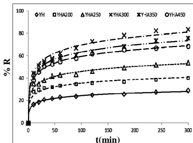
**Fig 2.** adsorption kinetics of MB molecule by YHx (x : activation temperature)
