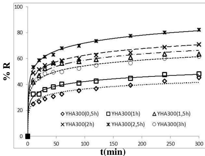
Fig 4. adsorption kinetics of MB molecule by YHA300t (t: the activation time)
