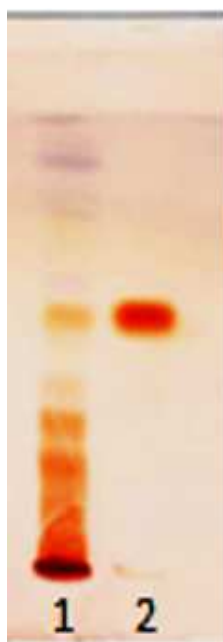
Fig.1. TLC profile of Sample solution of Saraca asoca stem bark 1: Sample solution; 2: (+)-Catechin standard
