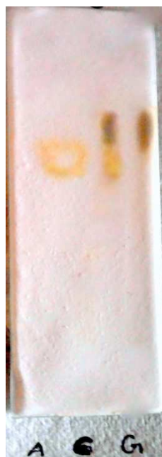
Figure 10: TLC studies of ascorbic acid Dichloromethane: Acetone: GAA (4: 3: 3) A – Ascorbic acid C – Ayurvedic Formulation G – Gallic acid
