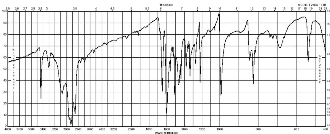
**Fig 3 FTIR spectra of 4-AP**
