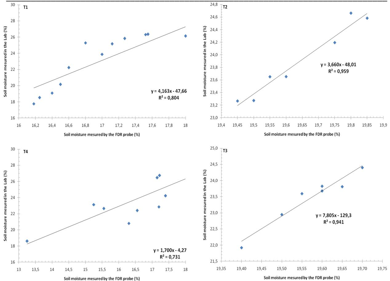
**Fig. 5 Correlation between Soil volumetric water content (%) obtained by the laboratory gravimetric method (Y) and that obtained in the field using FDR probe (X).**
