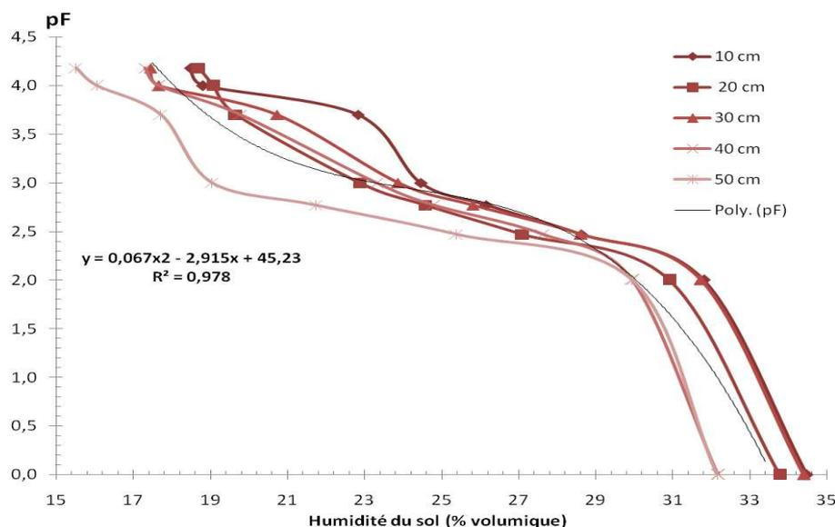
Fig. 2 Water retention curves (pF curves) for the experimental orchard
