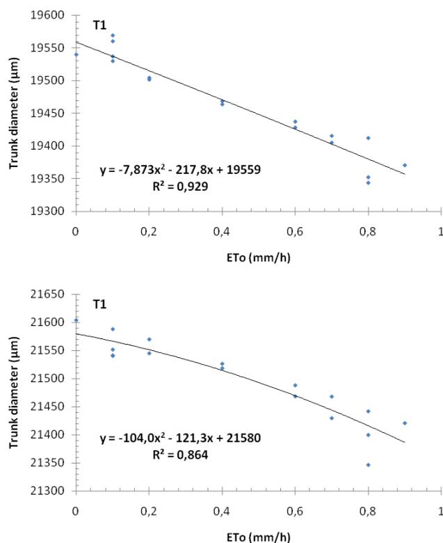
**Fig. 11** Correlation between trunk diameter measured using LVDT sensor, in relation to reference Evapotranspiration per hour (ETo), for Treatment 1 (dose = 1.05 mm/application and  $f = 10\%$ ).
