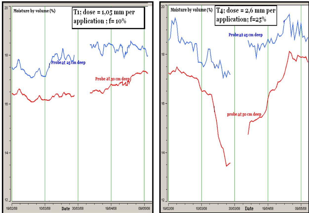
**Fig. 4** Changes in the soil volumetric water content, measured using FDR probe in T1 (very frequent applications of 1.05 mm/application ;  $f = 10\%$ ), and T4 (less frequent applications of 2.6 mm/application;  $f = 25\%$ ) for each of the two soil depths : 25 cm and 50 cm.
