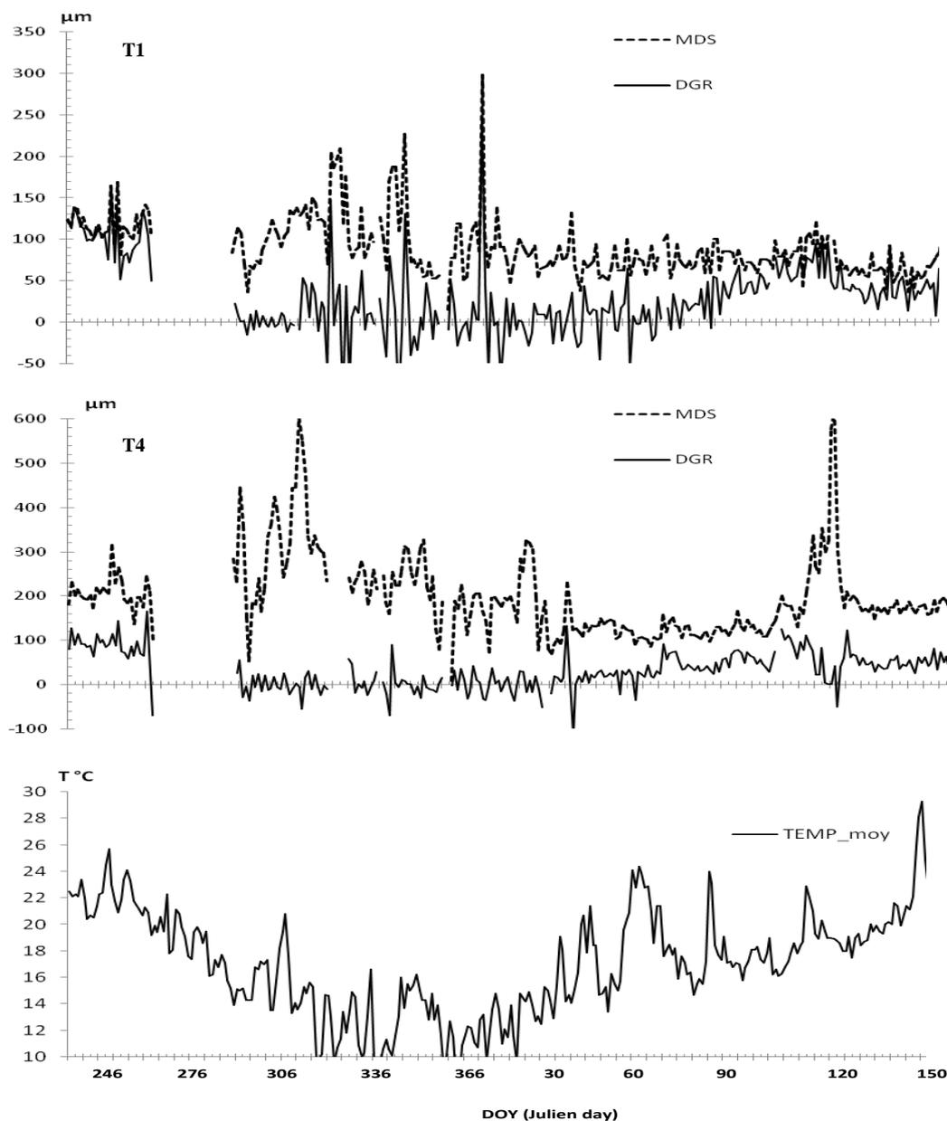
**Fig. 9** Maximum Daily Shrinkage (MDS) of the plant trunk and Daily Growth Rate (DGR) (using LVDT sensor), for Treatment 1 (dose = 1.05 mm/application and  $f = 10\%$ ) and Treatment 4 (dose = 2.6 mm/application and  $f = 25\%$ ) compared to the temperature average during 2010.
