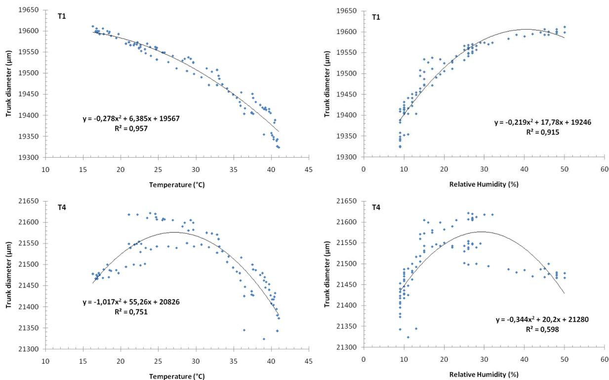
**Fig. 10** Correlation between trunk diameter measured using LVDT sensor, in relation to changes in temperature and relative humidity, for Treatment 1 (dose = 1.05 mm/application and f = 10 %).
