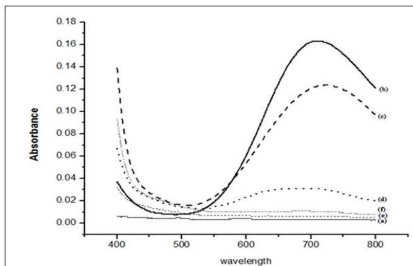
Figure 10: UV-Visible spectra of (a) RTB, (b) RTB+Cu, (c) RTB+Cu+AA at 5 min, (d) RTB+Cu+AA at 1 min, (e) RTB+Cu+AA, (f) RTB+Cu+AA at very high concentration
