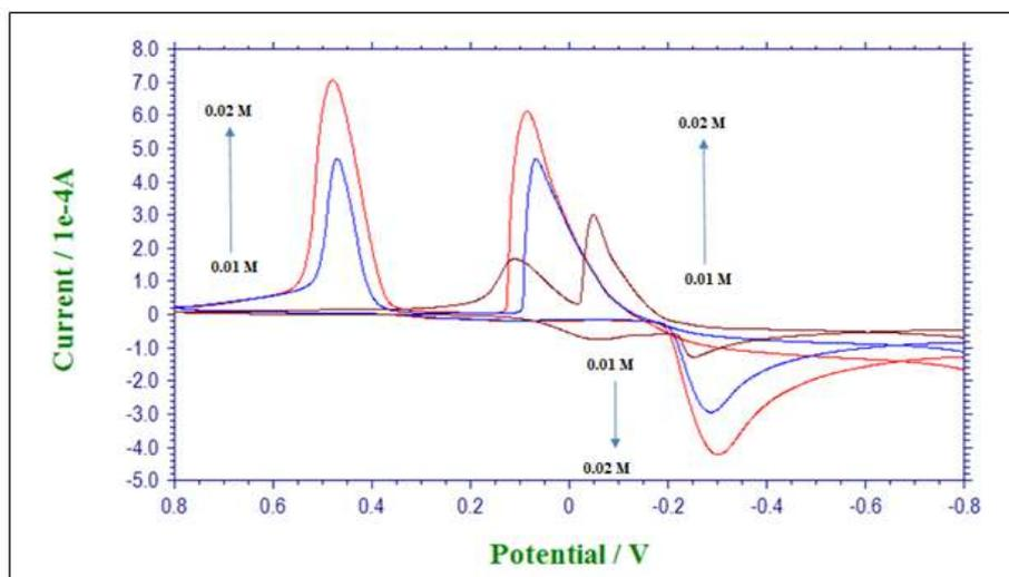
**Figure 4:** Cyclic voltammogram of 0.01 M and 0.02 M copper sulphate in presence of RTB in 0.1 M KCl
