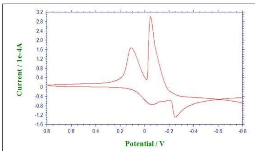
Figure 1: Cyclic voltammogram of 0.01 M in copper sulphate 0.1 M KCl
