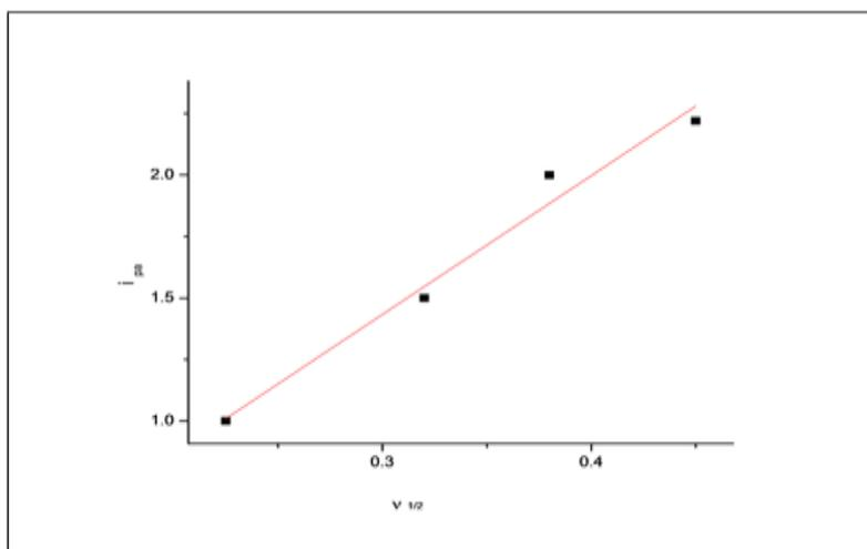
Figure 6: Plot of first cathodic peak current vs. square root of scan rate
