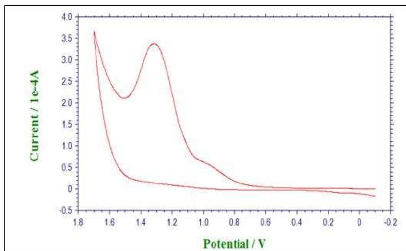
Figure 2: Cyclic voltammogram of 0.01 M in Rizatriptan benzoate in 0.1 M KCl
