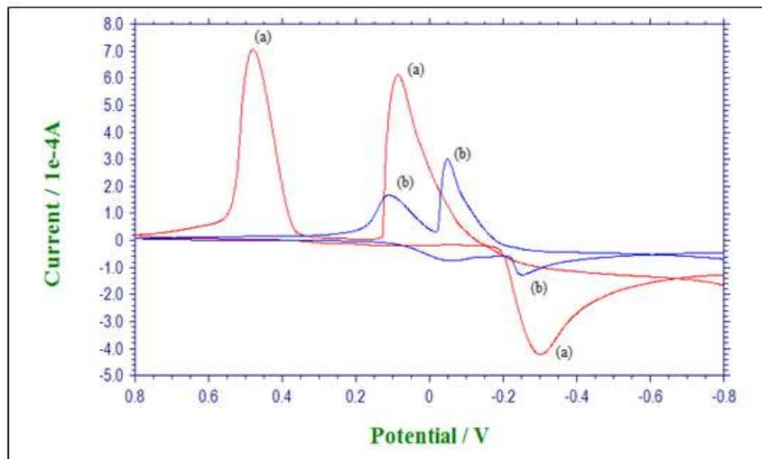
**Figure 3:** Cyclic voltammogram of (a) 0.01 M copper sulphate in presence of rizatriptan benzoate in 0.1 M KCl, (b) 0.01 M copper sulphate in 0.1 M KCl
