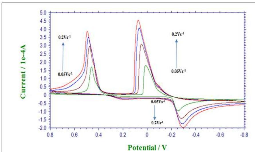
Figure 5: Cyclic voltammogram of 0.01 M copper sulphate in presence of RTB in 0.1 M KCl at different scan rates (0.05 Vs<sup>-1</sup>, 0.1 Vs<sup>-1</sup>, 0.15 Vs<sup>-1</sup> and 0.2 Vs<sup>-1</sup>)
