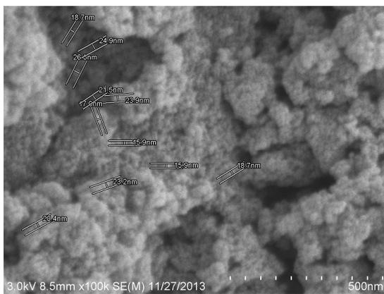
FIGURE 3 SEM image of the pure TiO<sub>2</sub>
