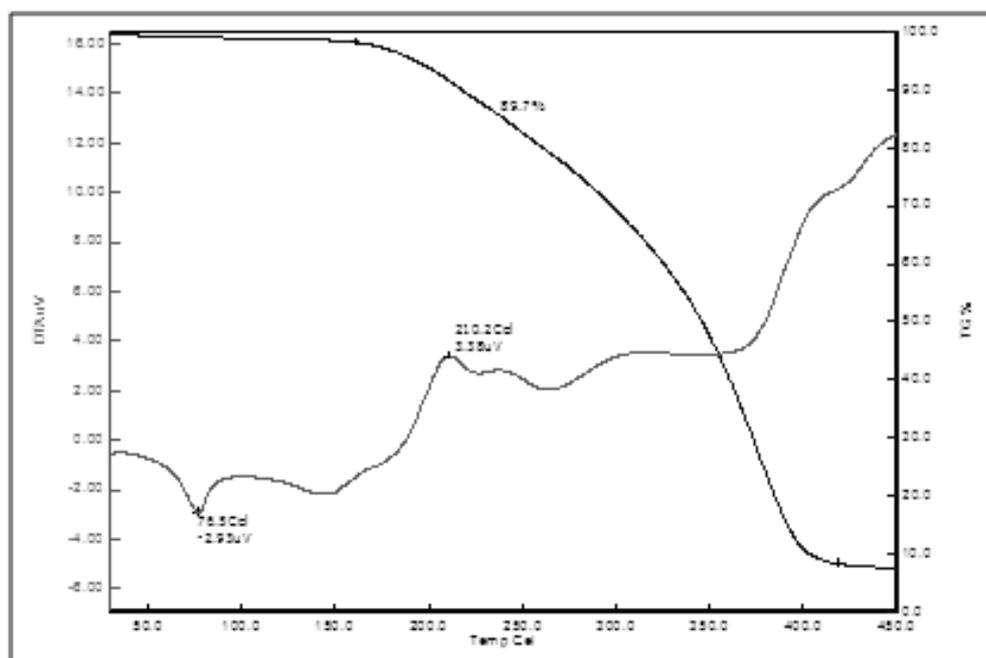
Fig.8 TGA-DTA curve of 2C4MBS
