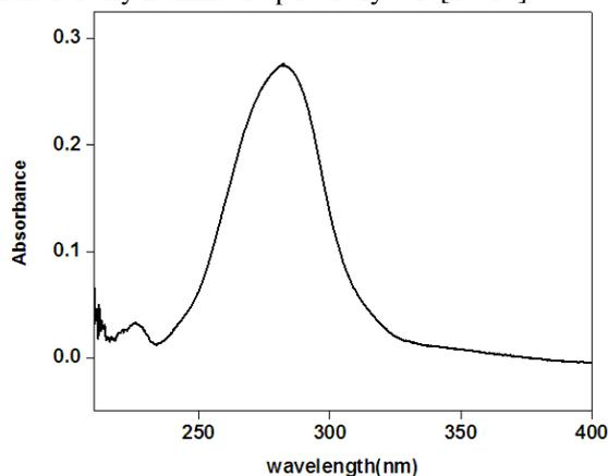
Fig. 6 UV spectra of 2C4MBS in acetonitrile
