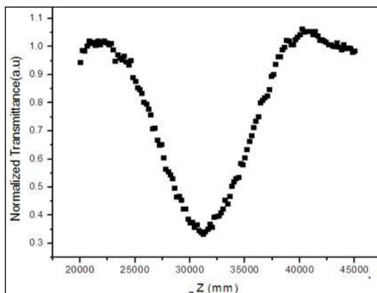
Fig. 7 Non linear absorption coefficient of compound 2C4MBS
