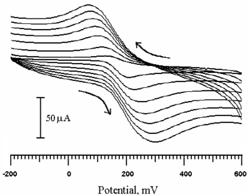
Figure.3a-Cyclic voltammogram of 1mM DA at different scan rate (50 to 300  $\text{mVs}^{-1}$ ) at TCPLMCPE in 0.2M phosphate buffer solution (pH 7.2).
