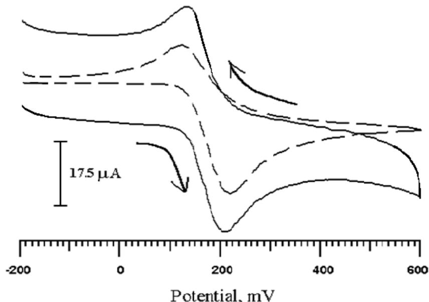
Figure.2-Cyclic voltammogram of 1mM DA in 0.2M phosphate buffer solution at pH 7 at BCPE (dotted line) and TCPLMCPE (solid line), at  $50 \text{ mVs}^{-1}$  in 0.2M phosphate buffer solution (pH. 7.2).
