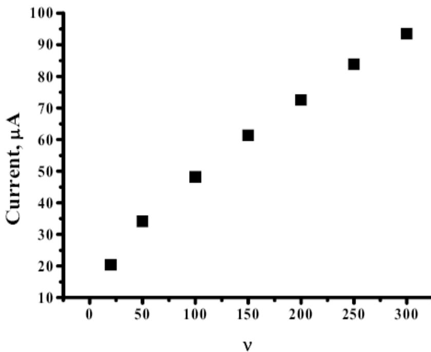
Figure.3b-Graph of current vs scan rate of DA.
