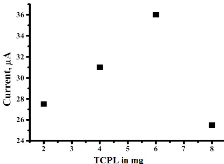
Figure.1-Graph of Ipa of DA vs different quantity of TCPL in carbon paste electrode.
