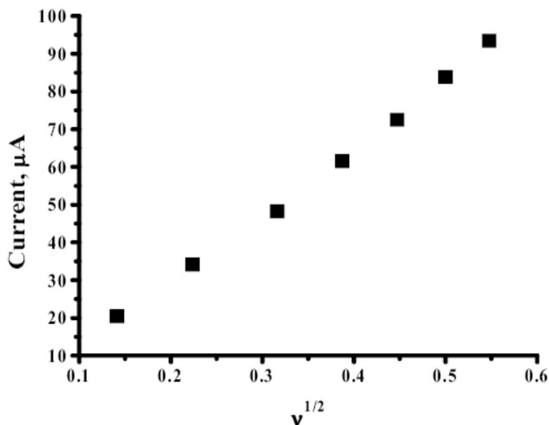
Figure.3c-Graph of current vs square root of scan rate of DA.
