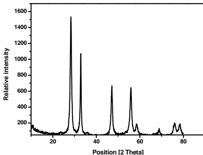
Figure 1 : The XRD patterns of the  $\text{Bi}_2\text{WO}_6$
