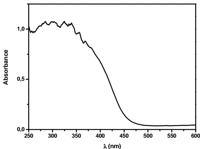
Figure 2: UV-vis diffuse reflectance spectra of  $\text{Bi}_2\text{WO}_6$
