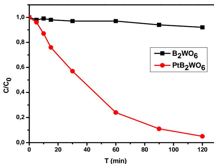
Figure 4: Photocatalytic removal of MO with  $\text{Bi}_2\text{WO}_6$  and  $\text{PtBi}_2\text{WO}_6$
