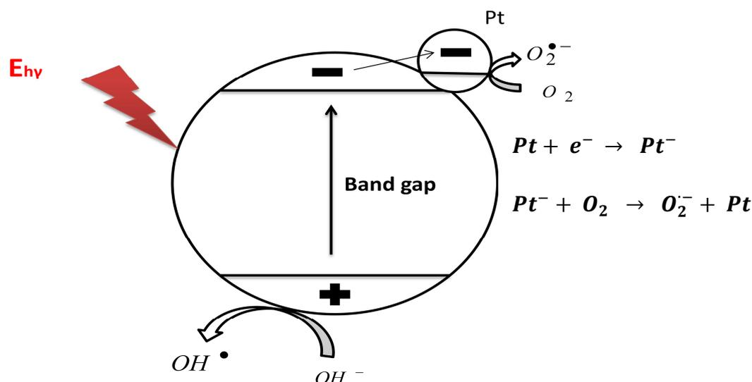
Figure 5: Schematic illustration of charge transfer process
