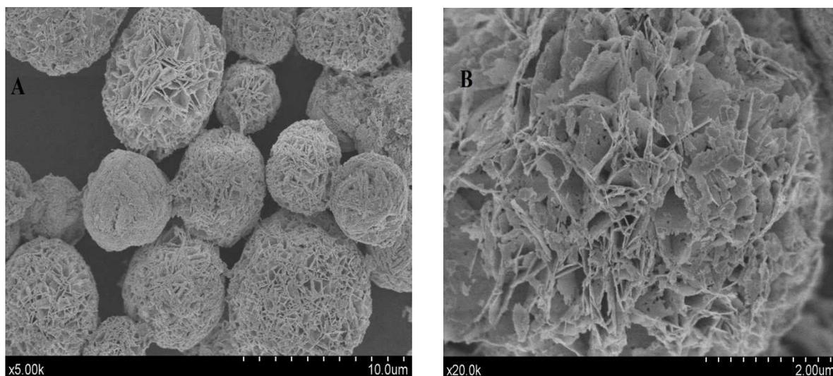
Figure 3: SEM images of  $\text{Bi}_2\text{WO}_6$ . (A): x5K; (B): x20K
