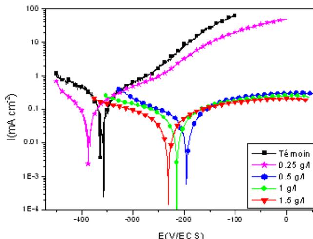
**Figure 6. Tafel polarization curves in HCl 1M with and without Elittaria Cardamomum oil at different concentrations at 298 K**
