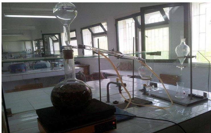
**Figure 3. Technical of hydrodistillation**
