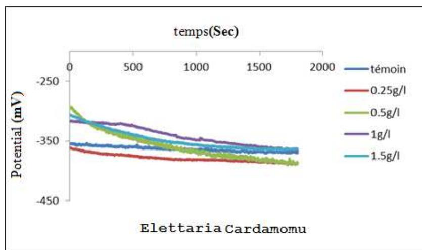
Figure 4. Potential change to the abandonment versus time brass in HCl 1M, with and without different essential oil concentrations studied at 298 K
