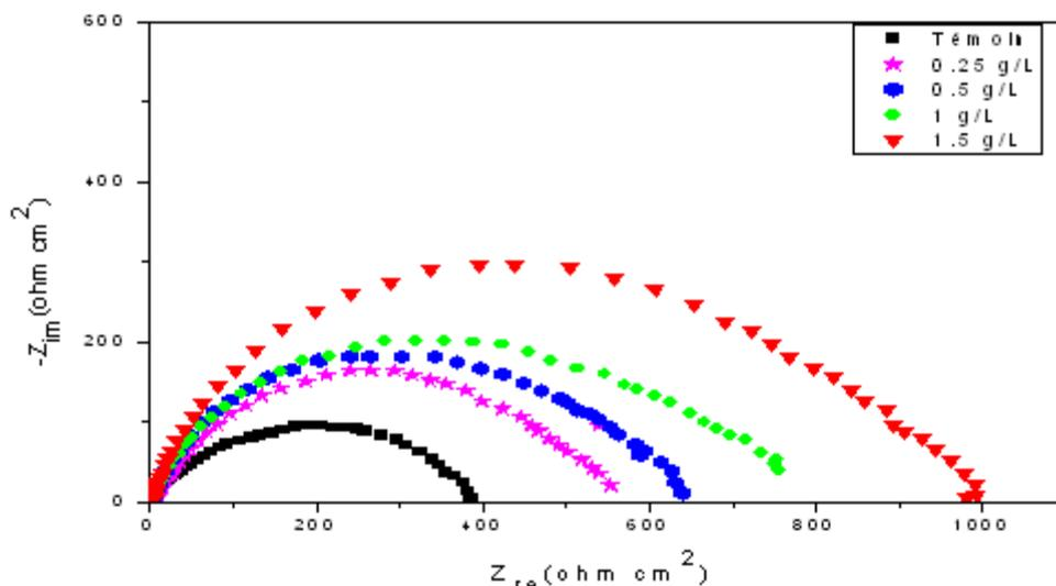
Figure 8. Nyquist plots in absence and presence of different concentrations of *Elettaria Cardamomum* oil in 1M HCl
