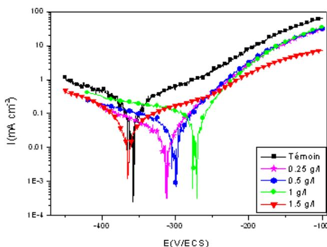
Figure 5. Tafel polarization curves in HCL 1M with and without *Nigella Sativa* oil at different concentrations at 298 K
