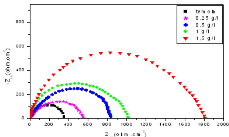
**Figure 7.** Nyquist plots in absence and presence of different concentrations of *Nigella Sativa* oil in 1M HCl
