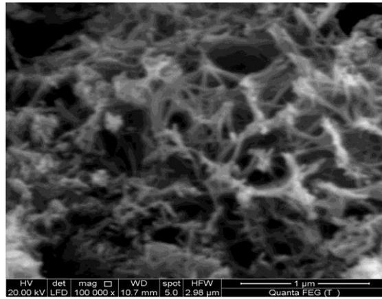
Figure 3b: FESEM image of H-Titanate Nanotubes (TNT)
