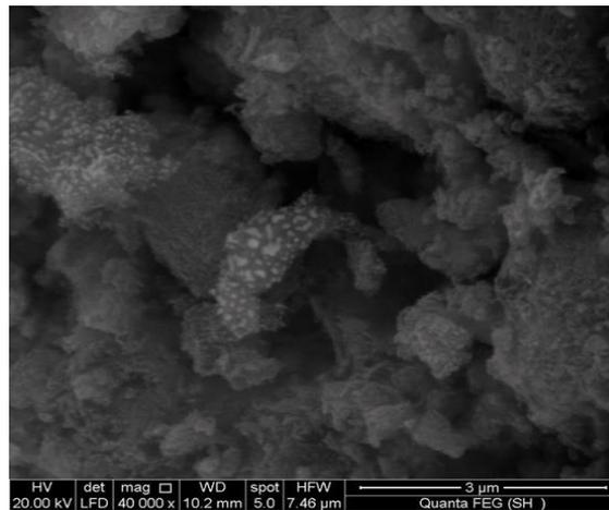
Figure 3c: FESEM image of multilayered H-Titanate Nanosheets (TNS)
