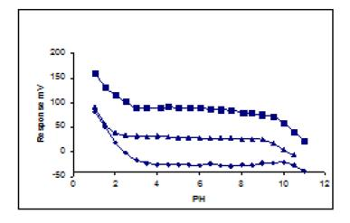
Figure 4: pH effect on CPH electrodes at different concentrations  $(\bullet \ 10^{-4}, \ \blacktriangle \ 10^{-3} \ \text{and} \ \blacksquare \ 10^{-2}) \ M$
