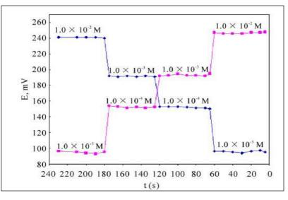
Figure 5: Response time for step changes in concentration of cyproheptadine hydrochloride
