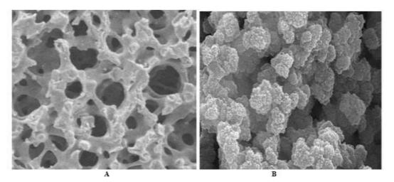
Figure 2: SEM photograph of the surface of MIP, (a) after washing, (b) before washing
