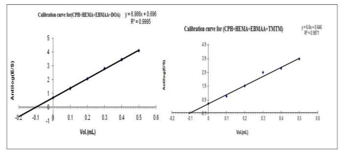
Figure 6: Calibration curve of estimation of cyproheptadine hydrochloride solution (10<sup>-3</sup>M) by MSAM using (CPH+HEMA+EBMAA+DOD, TMTM) electrodes
