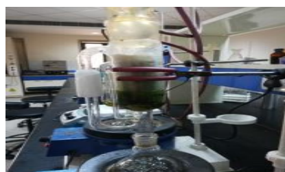
Figure 3: extraction of papaya leaves by soxhlet apparatus.
