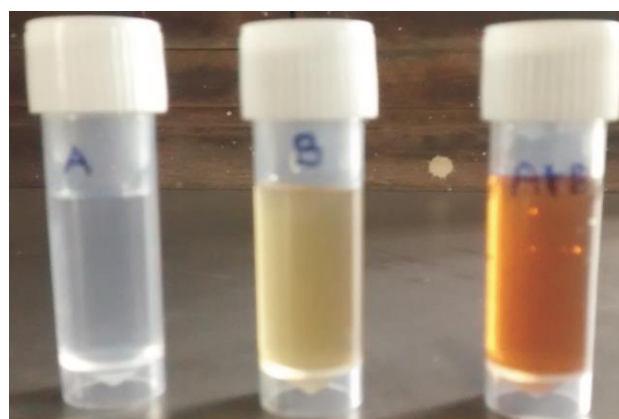
A - 10 mM \text{AgNO}_3 solution (before) B - Plant extract Averrhoa bilimbi (before) A+B - After synthesis \text{AgNO}_3 nanoparticles
