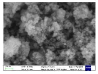
Figure 2: SEM image for NiFe<sub>2</sub>O<sub>4</sub> nanoparticles sintered at 500°C
