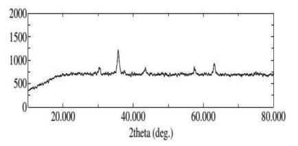
Figure 1: XRD patterns for NiFe<sub>2</sub>O<sub>4</sub> nanoparticles sintered at 500°C
