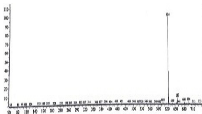
Figure 6: Mass spectrum of Zn(II) complex
