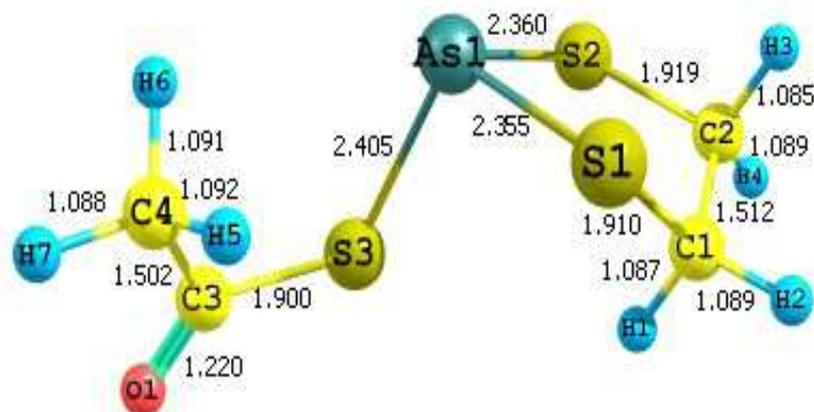
Fig.2. Optimized geometry of compound 2
