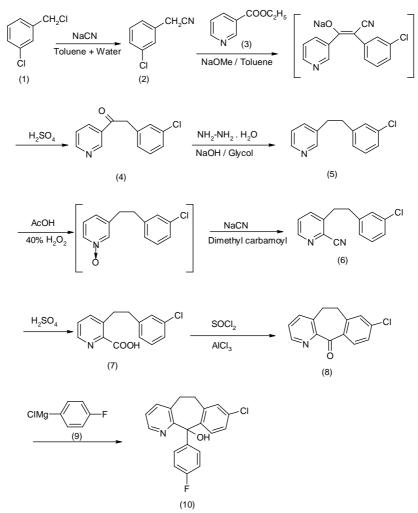
Scheme 1: Synthetic route for the preparation of Lead Compound (10) and its derivatives (10a-10e)
