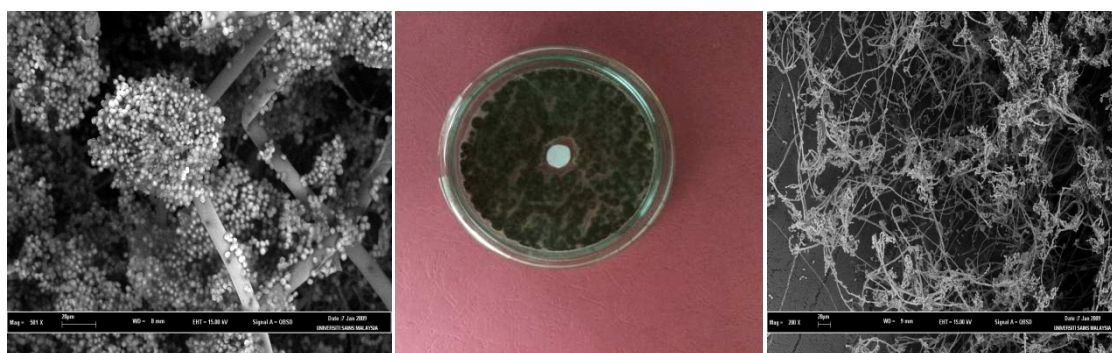
Fig 9. The morphology of Aspergillusniger : (a) before coated by TiO 2 -SiO 2 /chitosan (1:1) and (b) after coated by TiO 2 -SiO 2 /chitosan (2:1)
