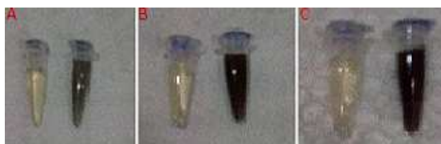
Fig. 1 Gold nanoparticles synthesized by endophytic fungi observed by colour change from pale yellow to pink. A) GX2-AuNPs B) GX3-AuNPs C) ARA- AuNPs
