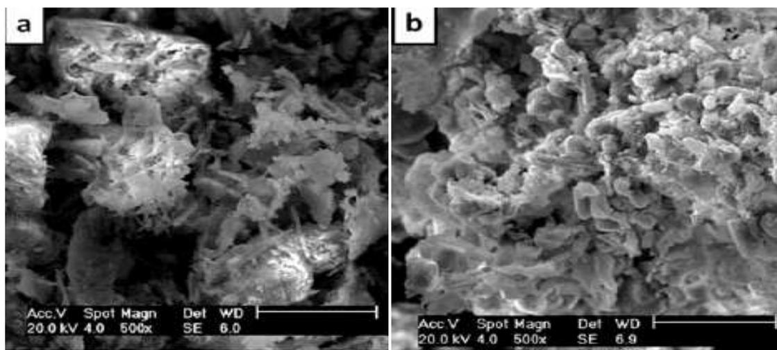
Fig.1: SEM image of Rice husk a: before used b: after used
