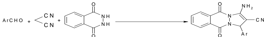
Scheme-II] One pot synthesis of pyrazolo [1,2-b] phthalazine dione
