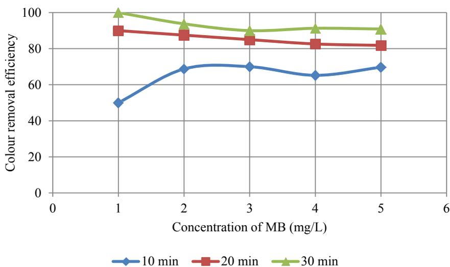
Figure 4: Graph showing relation between time and color removal efficiency
