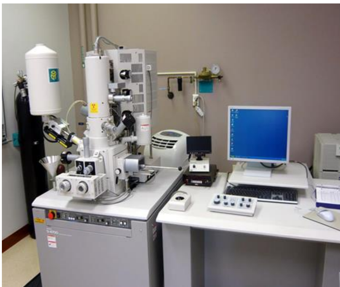
Figure 8a: Scanning electron microscope apparatus
